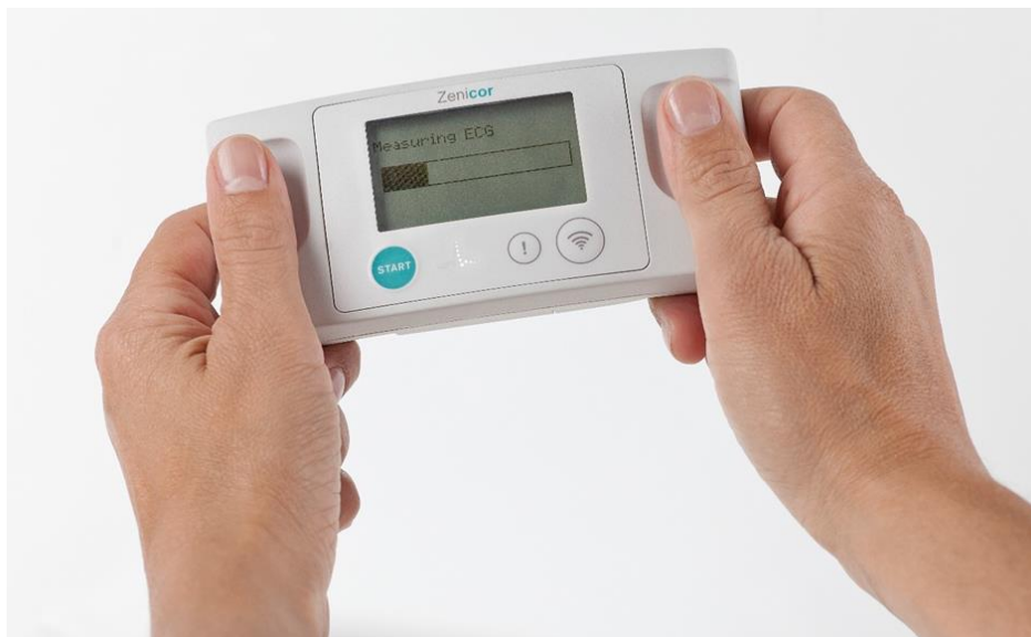
Figure 2 The Zeincor hand-held patient-activated lead-I electrocardiogram recorder, reproduced with permission from Zenicor®
