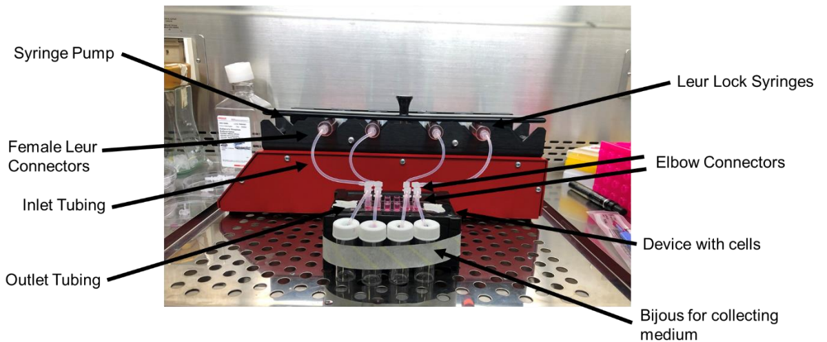
Figure 2.10 - Ibidi Device Experimental set up. Devices were connected to the syringe pump using female Luer connectors, inlet silicon tubing and elbow connectors. Elbow connectors were placed in the outlet and connected to silicone tubing in bijoux tubes to collect spent media for assays.
