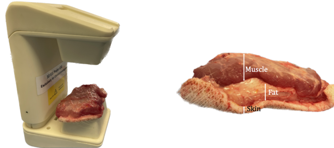
Figure 6.2: Photos showing the porcine tissue measured using the limb EIM device and the cross section of the tissue showing layers of skin, fat and muscle.
