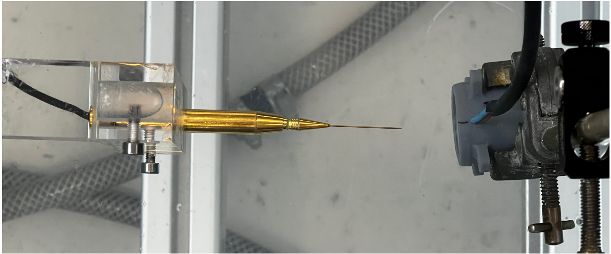
FIGURE 6.9: Hydrophone setup at the University of Glasgow used to measure the pressure field.
