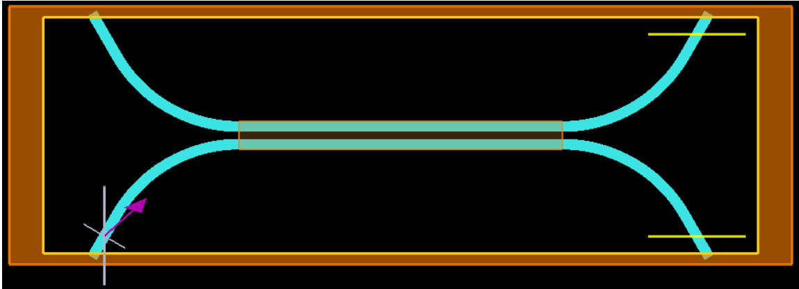
Figure 4.2. DC in FDTD. The blue material is the waveguide, the orange rectangle is the simulation region, the purple arrow is the input source, and the yellow lines are the detectors (y-normal cross transmission (upper right), y-normal parallel transmission (lower right) and z-normal field profile around the entire structure). The smaller orange rectangle around the coupling region is a higher-resolution mesh.
