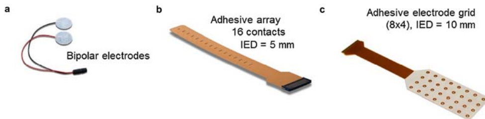
Figure 1.1.2 Surface electrode types in experimental signals. a Bipolar electrodes. b 1D electrode array. c 2D electrode array. Adapted from Journal of Electromyography and Kinesiology 49 , 102363 (2019) 17 .
