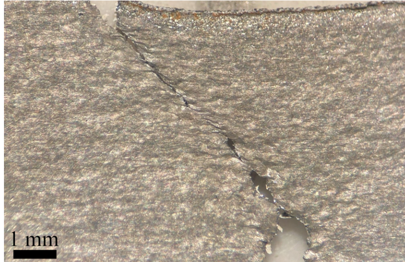
Figure 3.23: A micrograph of the rough texture developed during deformation.
