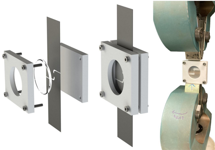
Figure 3.11: A render of the restraining system used for low triaxiality samples. Two plastic sections, one holding a sapphire glass window, are clamped around the sample. Right: Sample in tensile machine with applied restraint.
