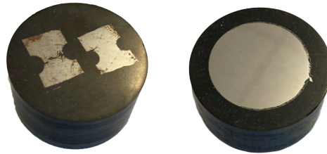
Figure 3.6: Samples mounted and polished for further characterisation. Left: Two notched samples from an interrupted tensile test. Right: A 0.2mm thick circle mounted for nanoindentation. The samples on the left have a fluorescent dye in the cracks and voids.
