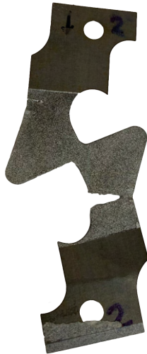
Figure 3.12: A sample which is not compatible with the restraint and fails outside of ROI.
