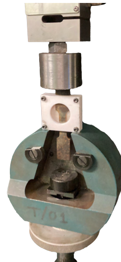
Figure 3.13: A test of frictional forces due to the restraining system. A sample is pushed through the clamped pieces.
