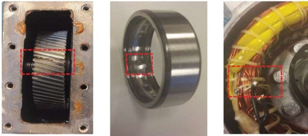
Fig. 6-2 Faulty components of electric powertrain: small gear tooth damage (left), Outer-race damaged bearing (mid) and 10% inter-turn short-circuit fault in the stator (right) [236].
