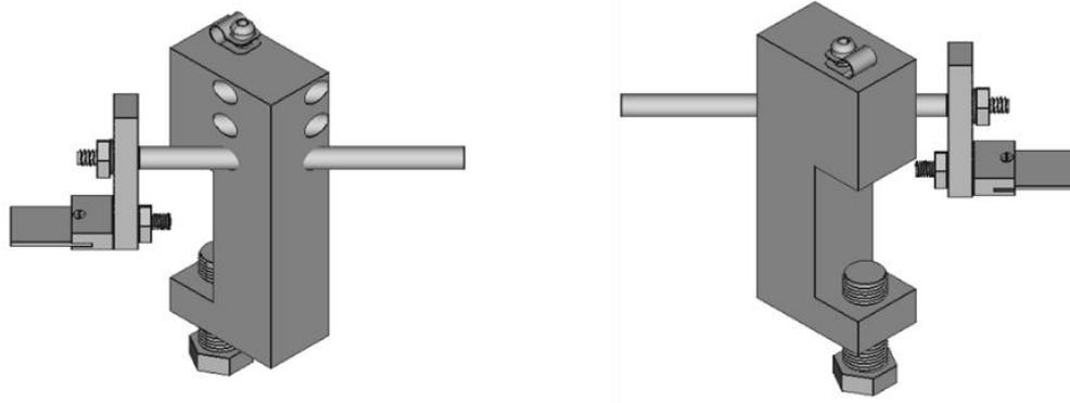
Figure 6.5.2 CAD drawings of the TEY detector.
