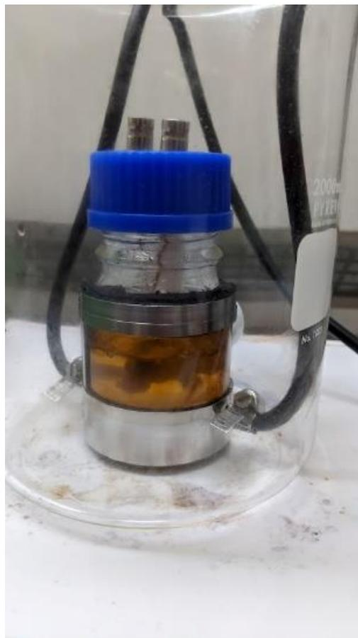
Figure 6.4.5 Experimental setup for in situ chemical treatment of the Cu foil.
