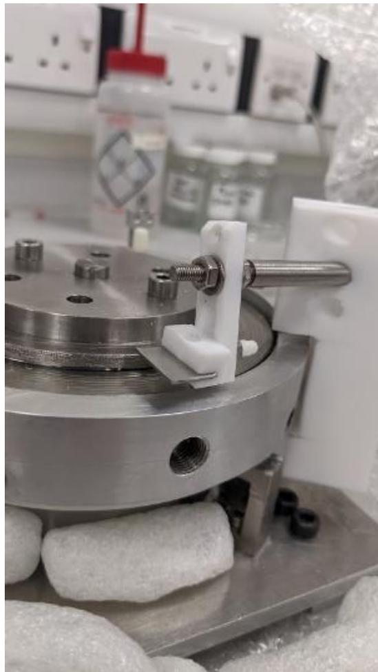
Figure 6.5.3 Image of the clamp assembly fixed on the side of the tribometer.
