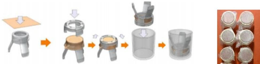
**Figure 3-3:** CellCrown™ transwell inserts are used to hold PCL fibres.
