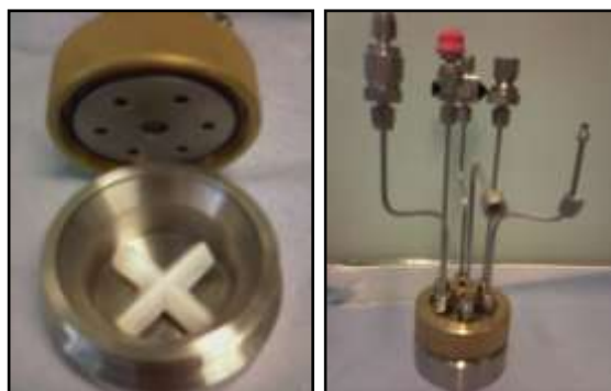
Figure 2.1: Stainless steel micro-reactor (49.0 cm 3 head space volume).
