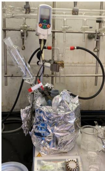
Figure 3.2 – The set-up for methacrylation step where an ice bucket, a dropping funnel, and a sheet of foil were set on the plate to set up a 0°C environment at 350 rpm in dark.
