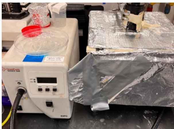
Figure 3.3 – OmniCure Series 1000, for curing the PGS-M scaffolds.
