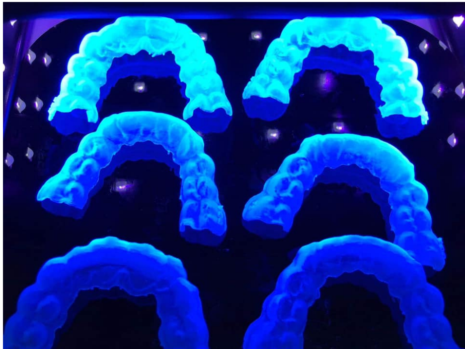
Figure 14. An Example of Direct-3D printed Aligners printed from STLs using an Asiga Max UV DLP 3D Printer and an experimental resin
