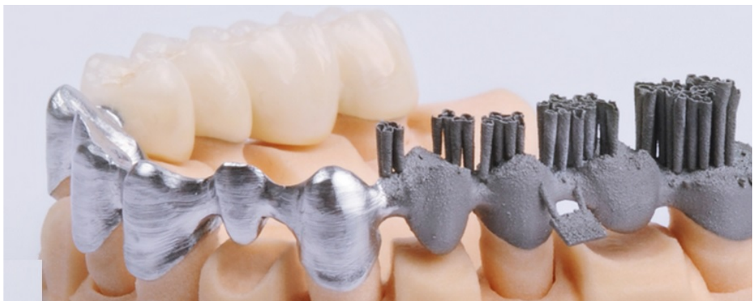
Figure 27. 3D Printed Metal Framework (Formlabs, 2019)
