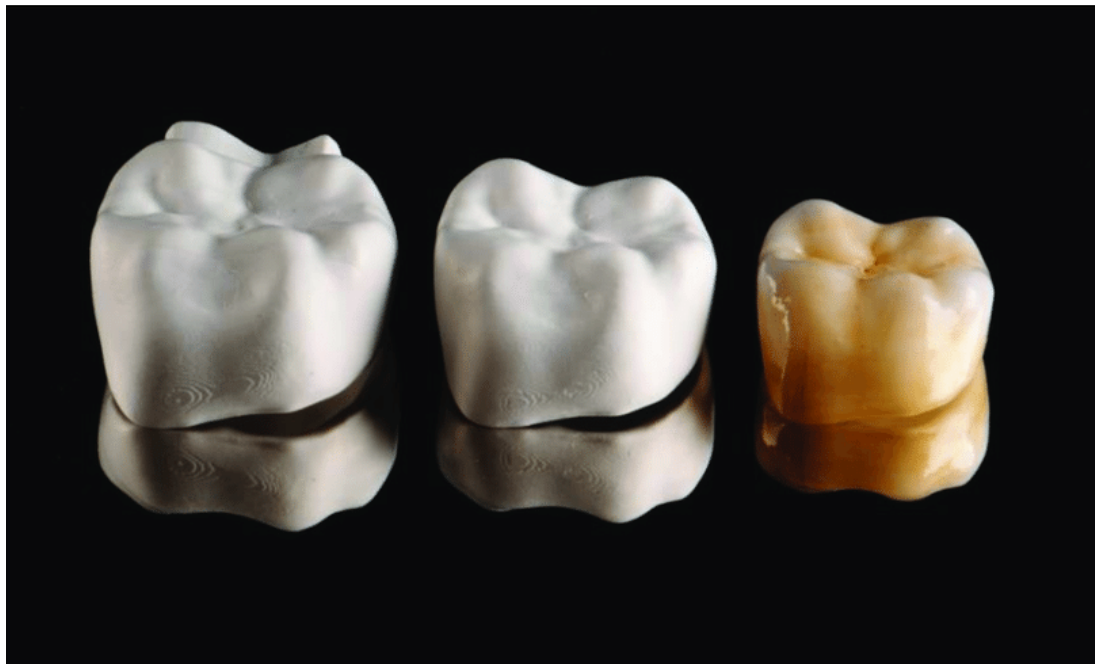
Figure 28. 3D Printed Zirconia Resin (Schweiger, 2021)
