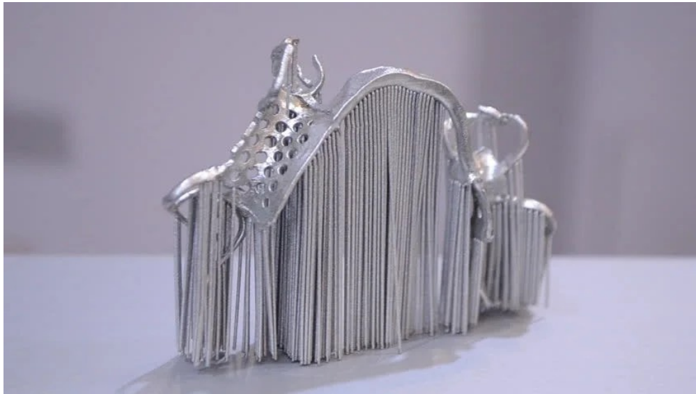
Figure 25. SLS 3D printed metal partial denture framework in CoCr (Formlabs, 2019)
