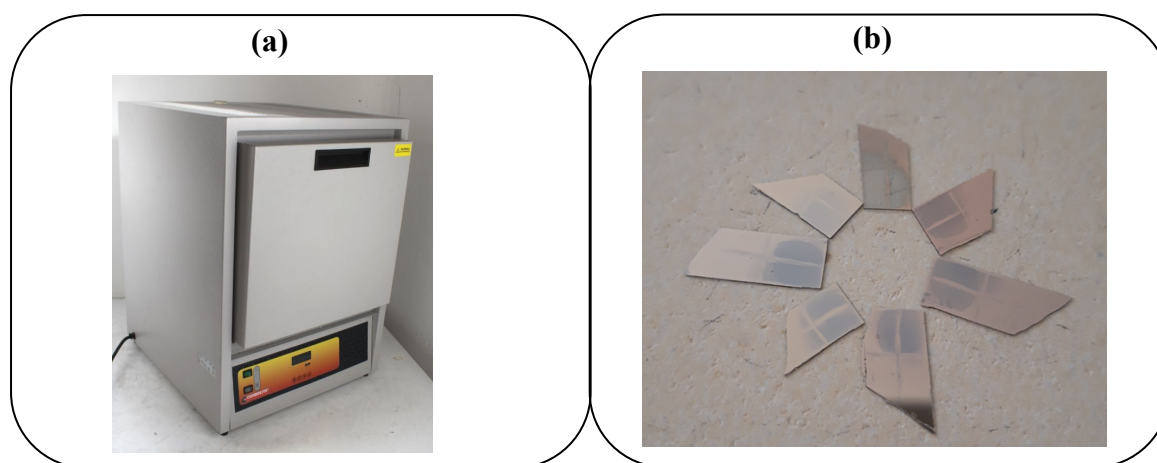
Figure 2.2. Photo of the carbolite chamber Furnace; and (b) the gold nanostructure samples inside the chamber furnace.
