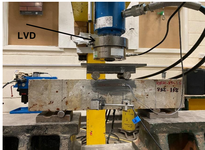
Figure 3.16: Details of the flexural strength tests using the short prismatic beams
