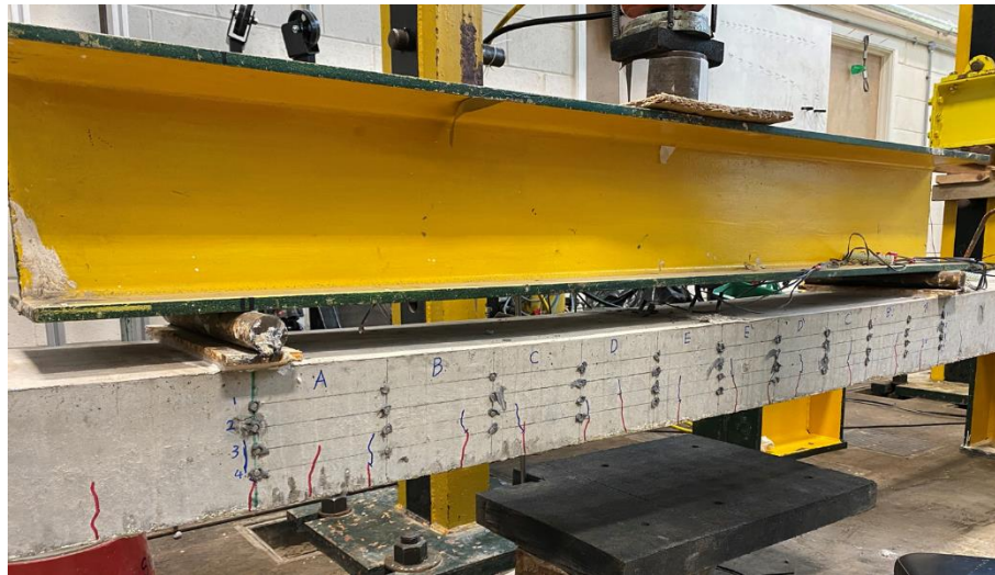
a) Visual examination of the crack pattern
