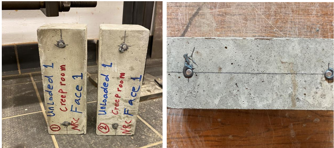
Figure 3.12: Shrinkage test specimen
