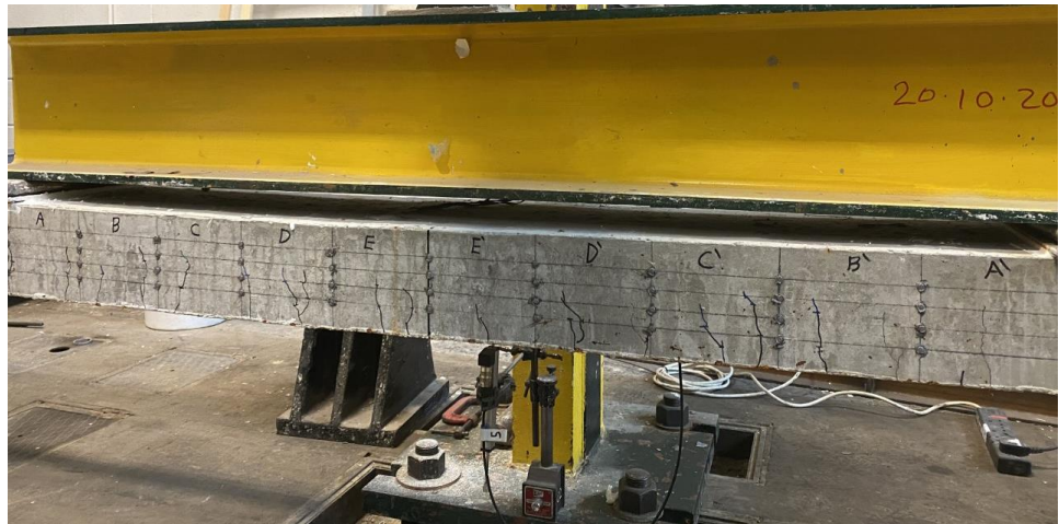
a) The final crack pattern of the experimental results before the failure occurred
