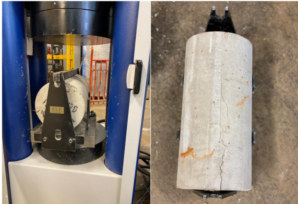
Figure 3.10: Splitting tensile strength test
