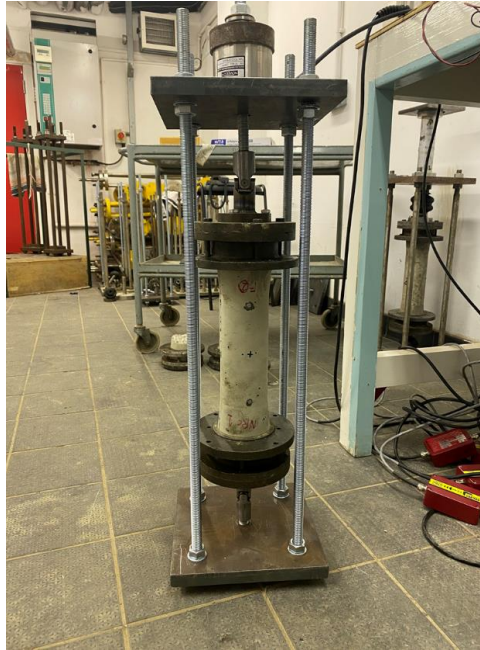
Figure 3.14: Tensile creep test set up
