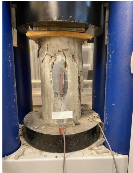
Figure 3.11: Test set up for measuring modulus of elasticity
