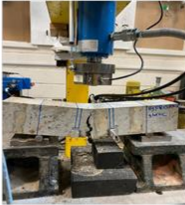
Figure A.18: The final crack pattern of the experimental results at the failure
