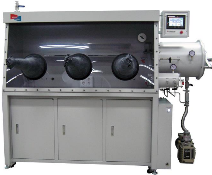
Figure 3.7 KOREA KIYON glovebox system
