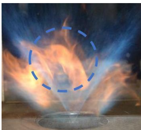
Figure 6-8 Direct image of a steady heptane swirl flame studied with a solid-cone spray atomizer.
