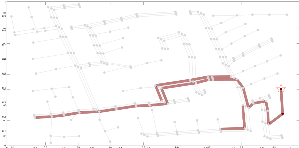
Figure K.11: Representation of M^P and M^Q values obtained for values higher than 0.5 when there is a single-phase perturbation at node 85, phase C. Load consumption with a rated power of 400 kW and 200 kVAR. (Scenario S1)
