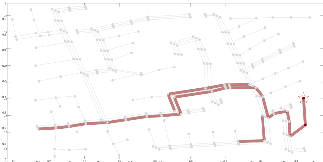
Figure K.12: Representation of M^P and M^Q values obtained for values higher than 0.5 when there is a single-phase perturbation at node 85, phase C. Photovoltaic generation with a rated power of 400 kVA at unity power factor. (Scenario S2)
