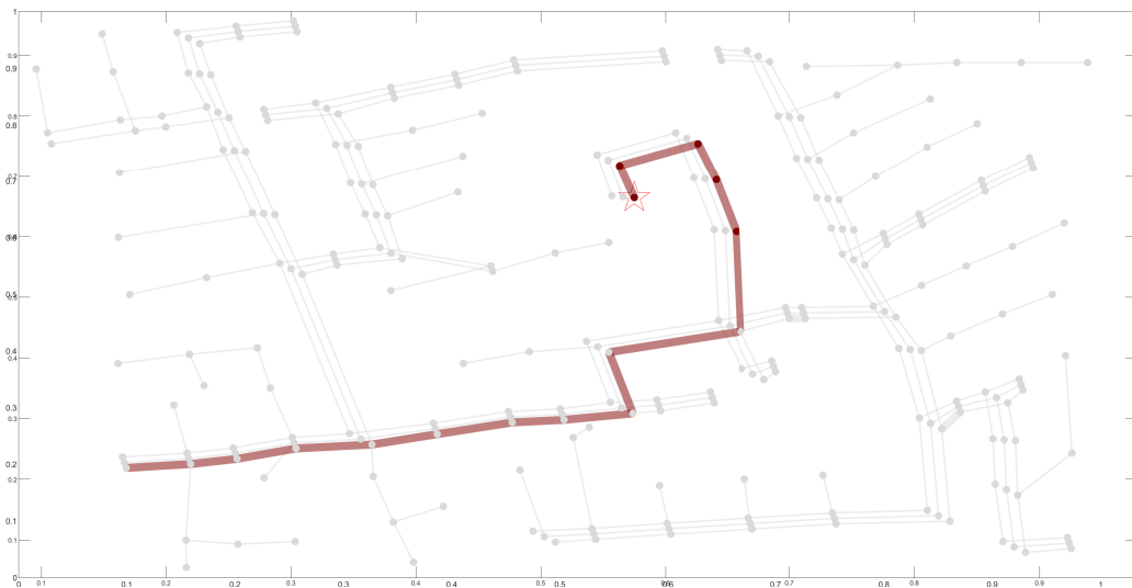
Figure K.3: Representation of M^P and M^Q values obtained for values higher than 0.5 when there is a single-phase perturbation at node 66, phase C. Load consumption with a rated power of 400 kW and 200 kVAr. (Scenario S3)
