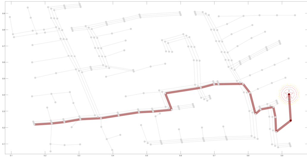
Figure K.2: Representation of M^P and M^Q values obtained for values higher than 0.5 when there is a single-phase perturbation at node 85, phase C. Photovoltaic generation with a rated power of 400 kVA at unity power factor. (Scenario S2)
