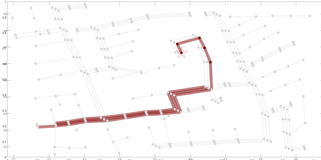
Figure K.8: Representation of M^P and M^Q values obtained for values higher than 0.5 when there is a single-phase perturbation at node 66, phase C. Load consumption with a rated power of 400 kW and 200 kVAr. (Scenario S3)
