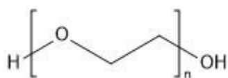
Figure 1.4: Chemical structure of PEG, with the non polar moiety shown as the two (CH 2 ) 2 groups within the repeating O(CH 2 ) 2 unit
