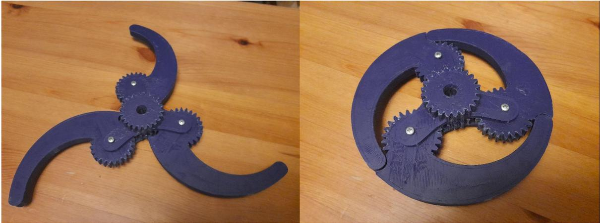
Figure 54. Initial Whieg design, physical. On the left with legs deployed and on the right as a wheel.
