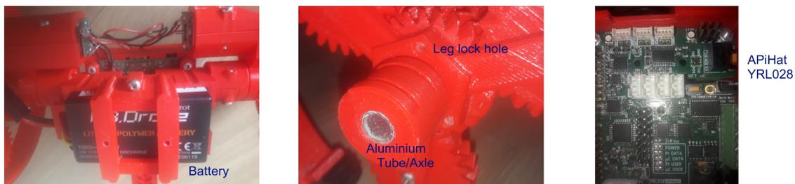
Figure 78. Battery housing, Aluminium tube axle/leg lock and APiHAT
