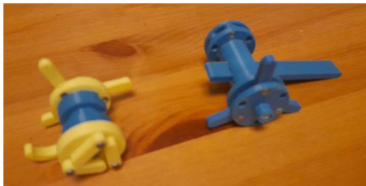
Figure 50. Scale models. On the left version one with exterior legs and a curved tail. On the right, version 2 which has the legs in a wheel sandwich and a straight tail.
