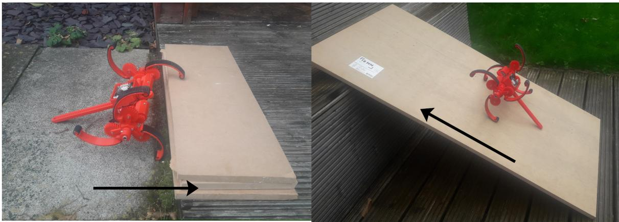
Figure 86. Physical experiment setup. For the step 2 cm/1 cm thick planks were used to adjust height. The same material was used against a bench and slotted decking for the slope. The fixed height increments and slotted decking mean repeatability of the environment was not an issue. Arrows show direction of travel.
