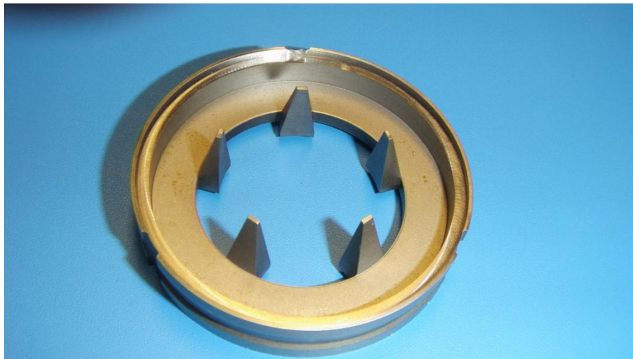
(a) One set of SMC claw-pole stator
