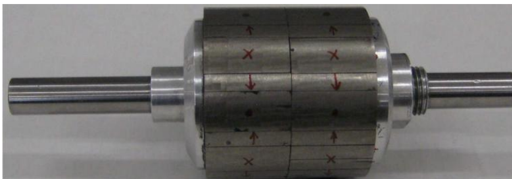
(a) Rotor with 2-segment Halbach array ( R_{mp}=0.7 )
