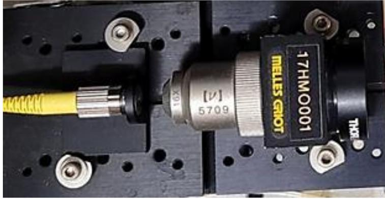
Figure 7.2: Fibre launch block with input/output optical fibre (left) a 16x magnification (11mm focal length) objective on a three-axis adjustable optical block.
