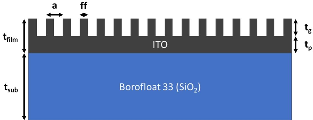
Figure 4.12: Schematic of 1D periodic structure in ITO showing some of the parameters that need to be known: substrate thickness ( $t_{sub}$ ), film thickness ( $t_{film}$ ), grating thickness ( $t_g$ ), waveguide thickness ( $t_{wg}$ ), grating period ( $a$ ), and grating fill factor ( $ff$ ).
