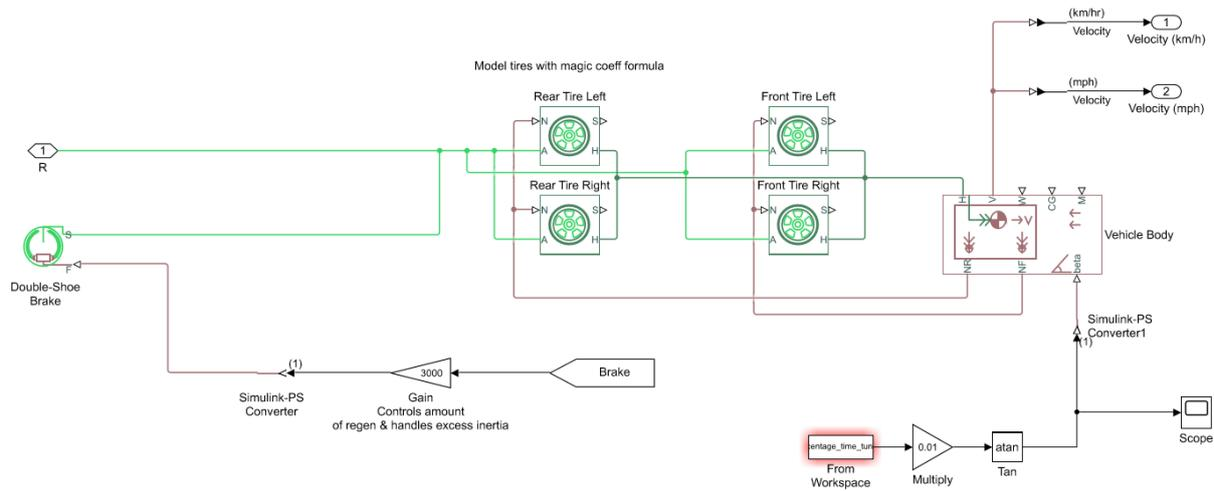
Figure 3.11 - Aerodynamic & brake subsystem models
