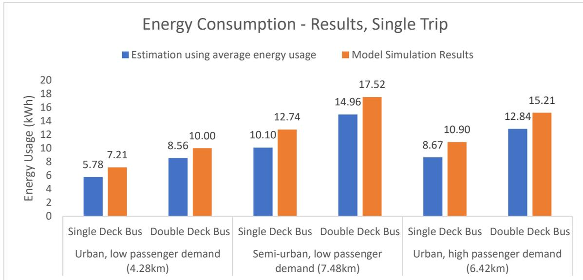
Figure 5.10 - Energy consumption results - simulated telemetry
