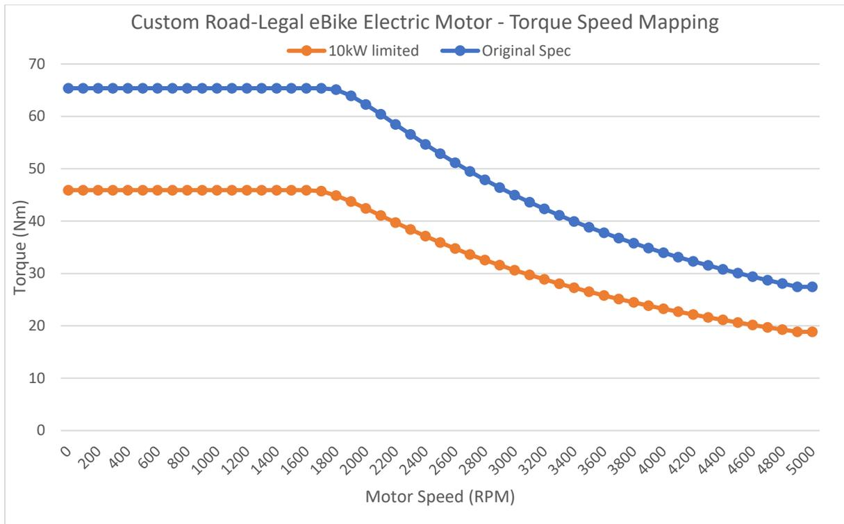
Figure 6.11 - Torque-speed map of presented motor spec
