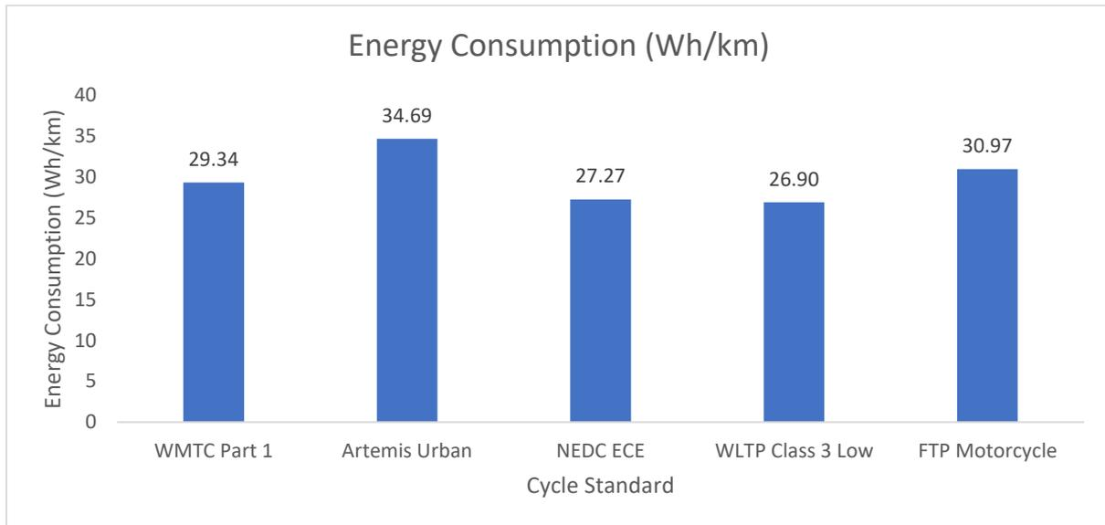
Figure 6.15 - Normalised energy consumption from simulation results
