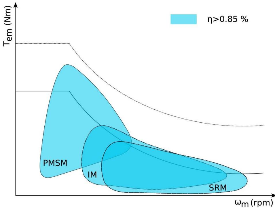
Figure 2.9 - Performance range and efficiency of various electric motor types [84]
