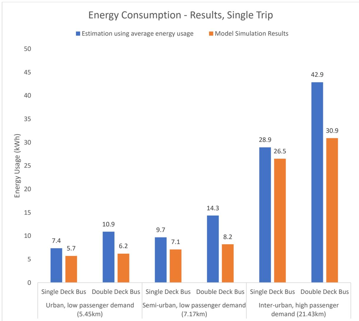
Figure 5.15 – Simulation results – real-life telemetry
