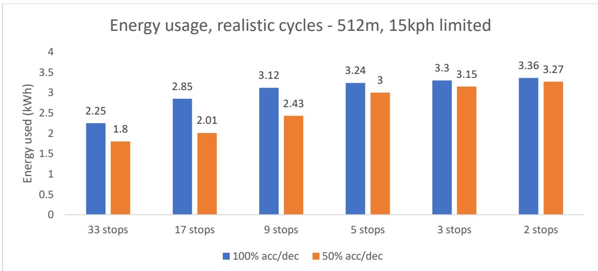
Figure 5.29 - Realistic cycle driving pattern comparison, various acceleration intensities
