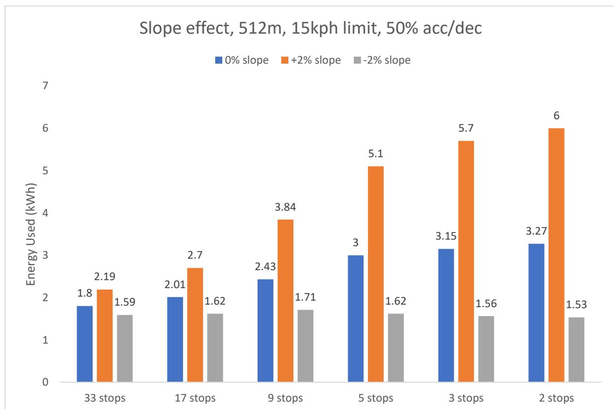
Figure 5.30 - Realistic cycle driving pattern comparison, various number of stops and slope variations
