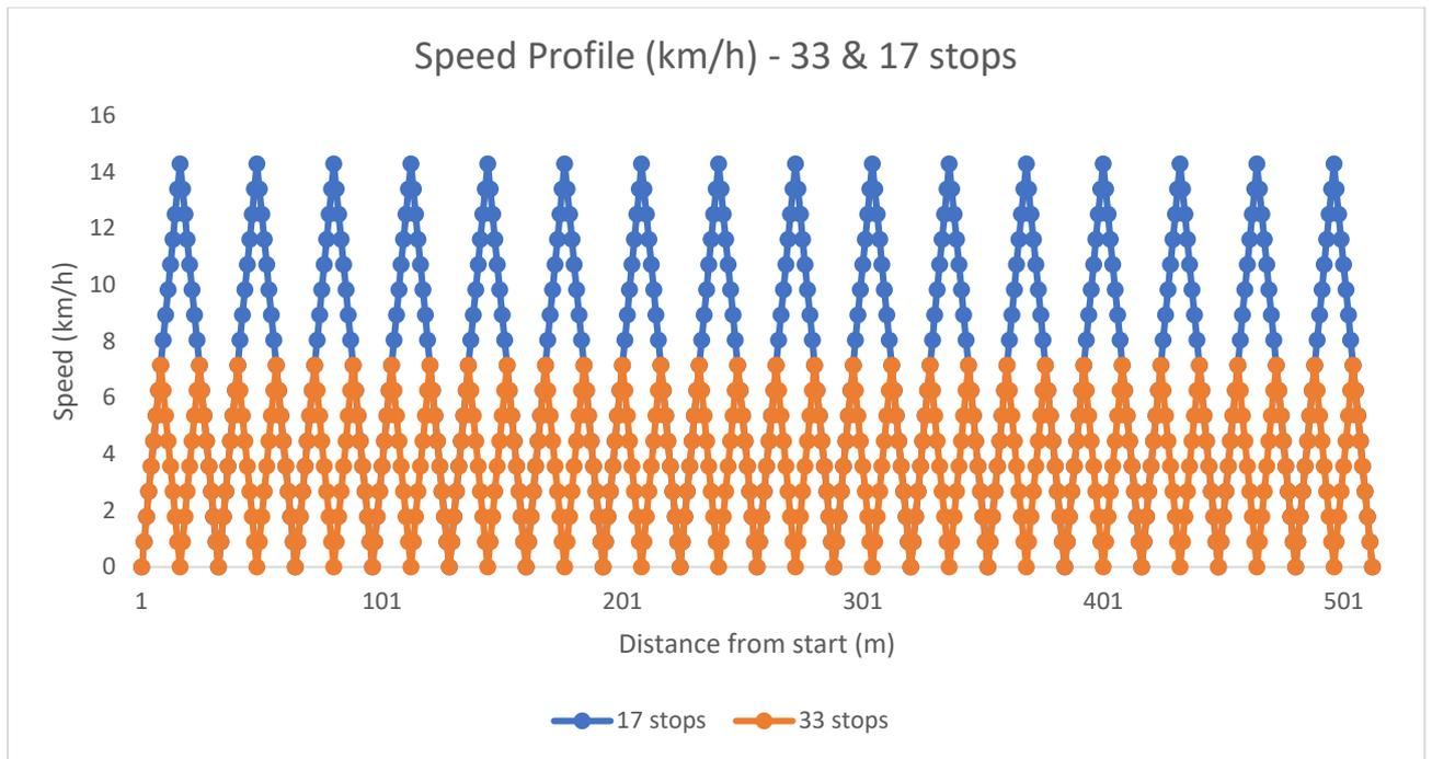
Figure 5.26 - Realistic cycle driving patterns. 33 & 17 stops, 512m street, 20kph limited
