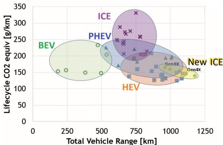
Figure 2.12 - Carbon Dioxide emissions vs vehicle range for different powertrain technologies. (Source: 27th Aachen Colloquium Automobile and Engine Technology, 2018)
