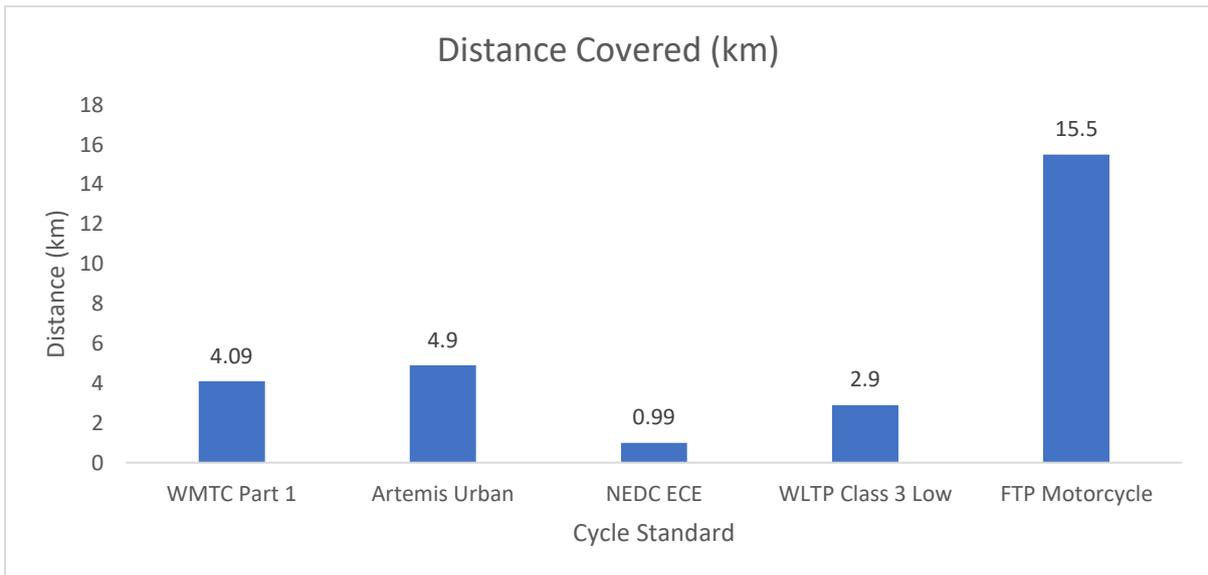
Figure 6.14 - Covered distance for every driving cycle in the input dataset
