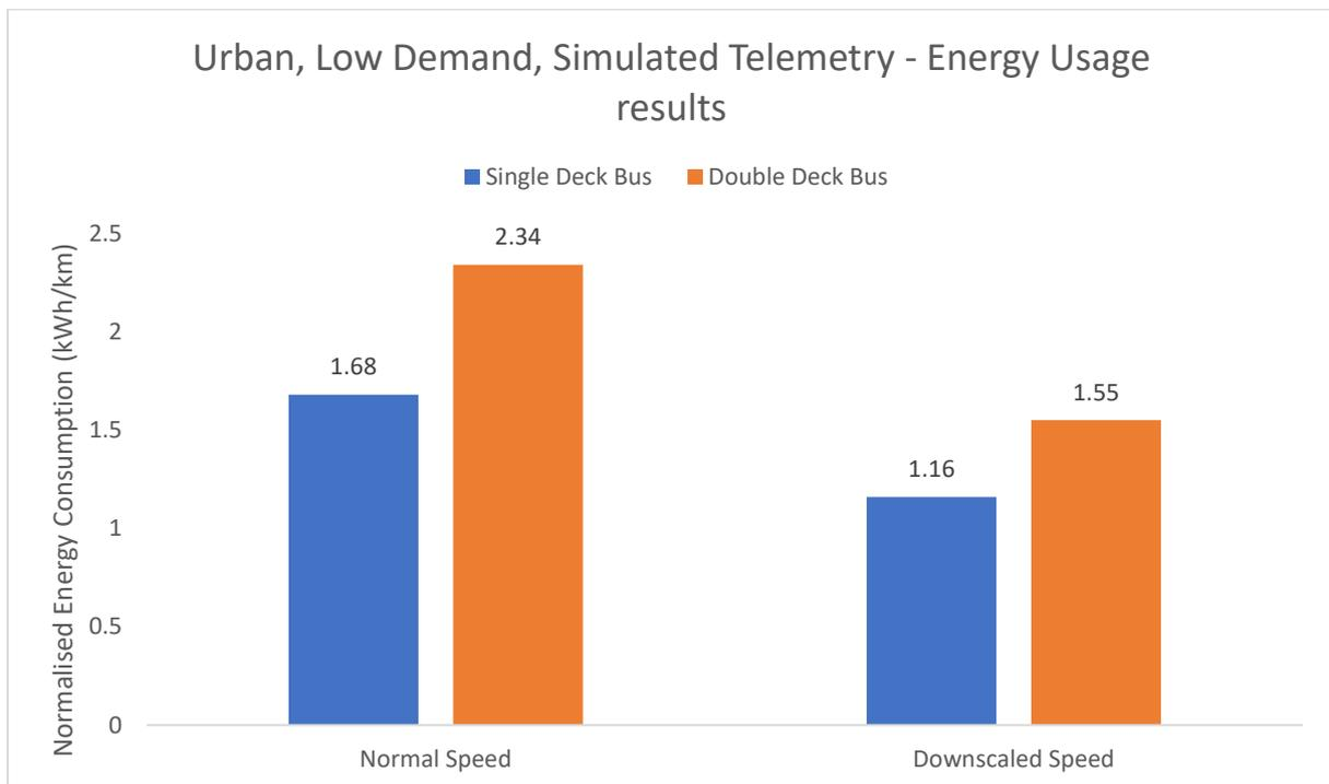
Figure 5.18 - Energy usage (normalised) comparison between normal simulated telemetry and downscaled version
