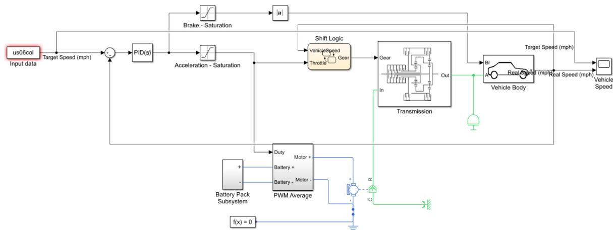
Figure 3.2 - Modelling approach employed by the first vehicle model iteration
