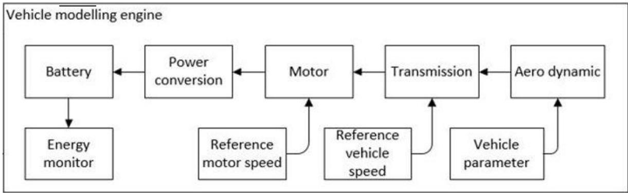
Figure 3.4 - Vehicle model, system block diagram
