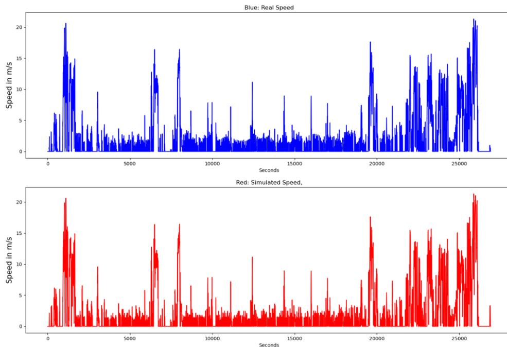
Figure 4.2 - Real driving data vs simulated cycle generated by emulation code
