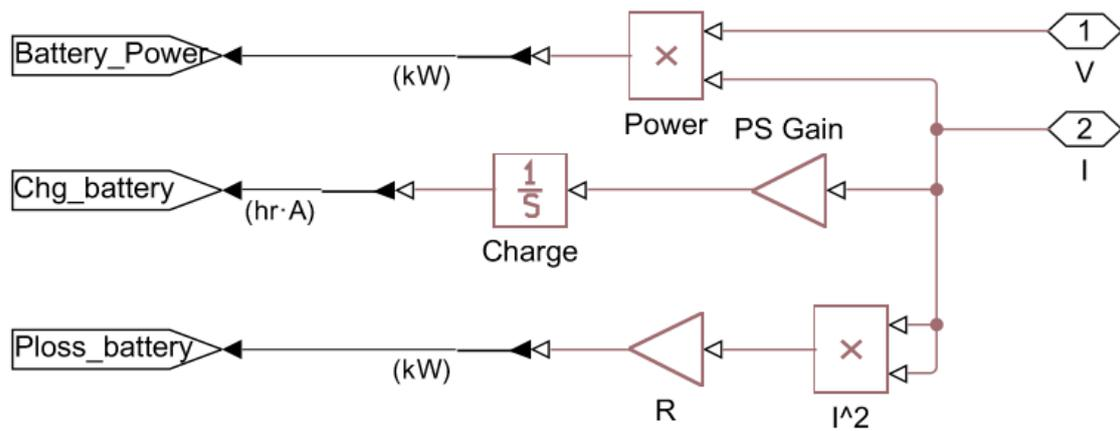
Figure 3.6 - Battery charge monitoring subsystem
