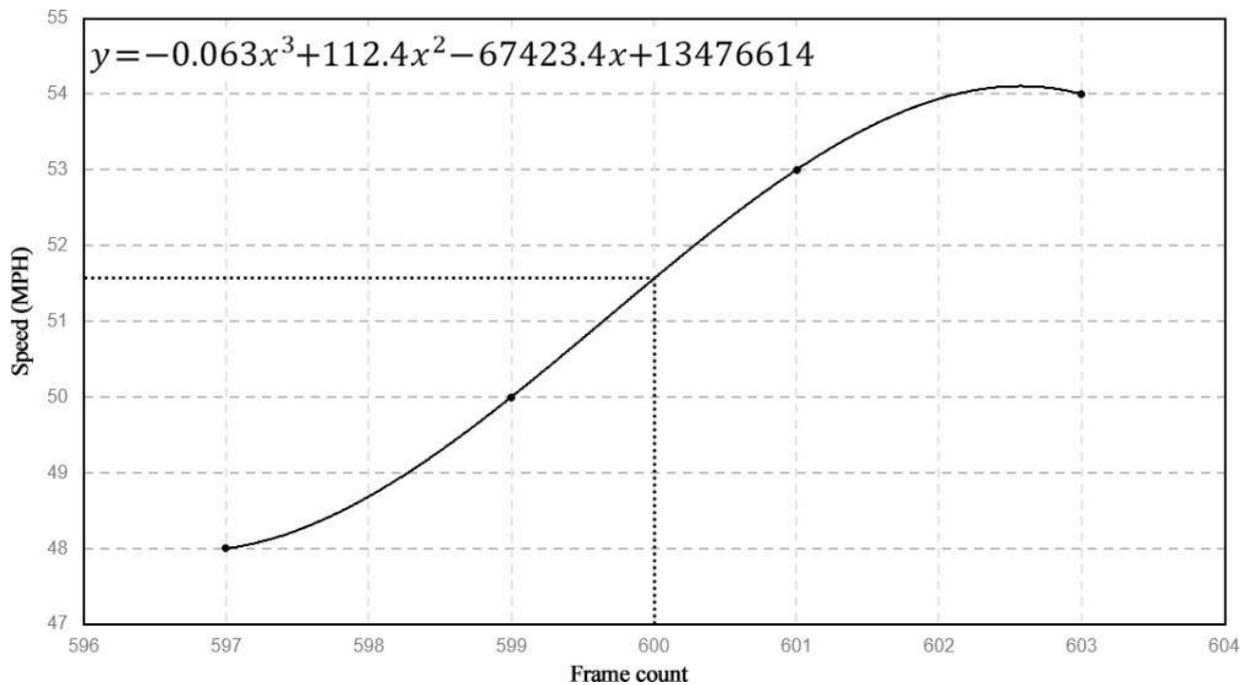
Figure 6.4 - A plot of the polynomial approximation for OCR results of the frame group presented in figure 6.5. The mathematical equation described by the curve is shown on the top-left side of the image
