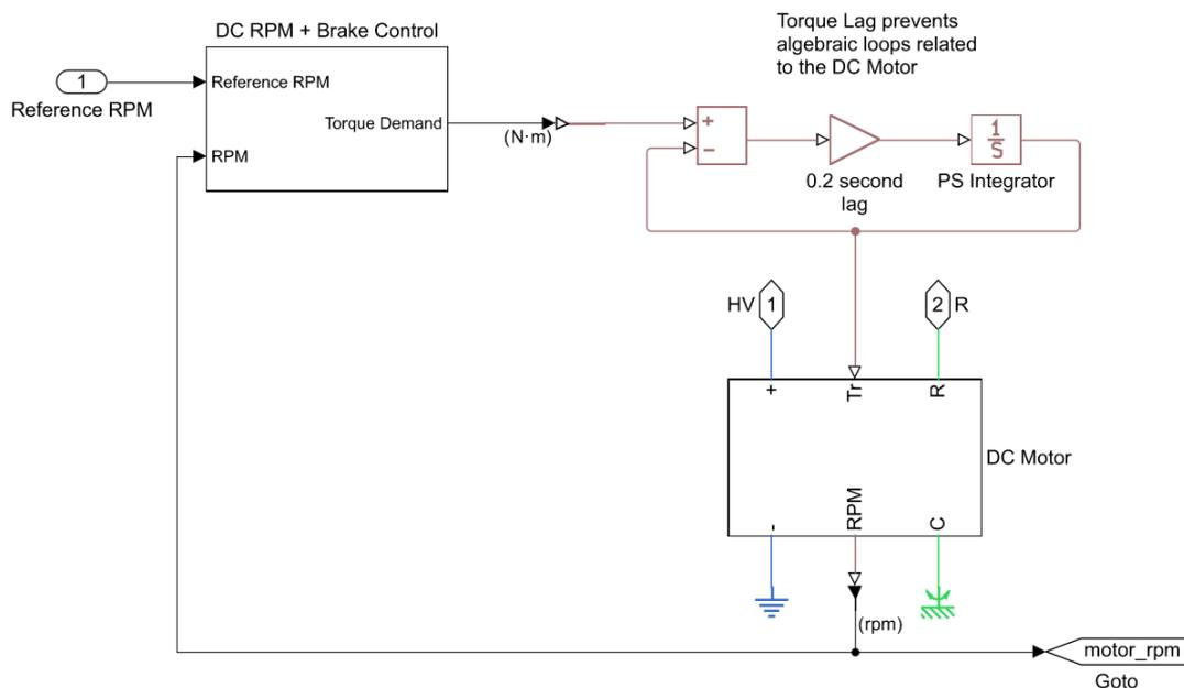
Figure 3.7 - DC motor + motor control subsystems
