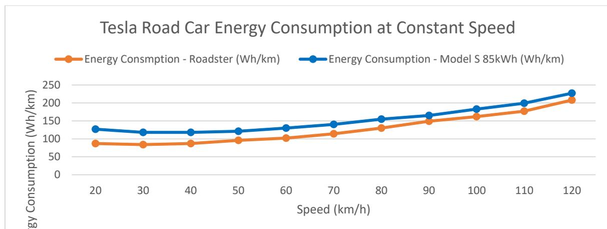
Figure 7.1 - Energy consumption curve for Tesla EV models. Source: Tesla Inc.
