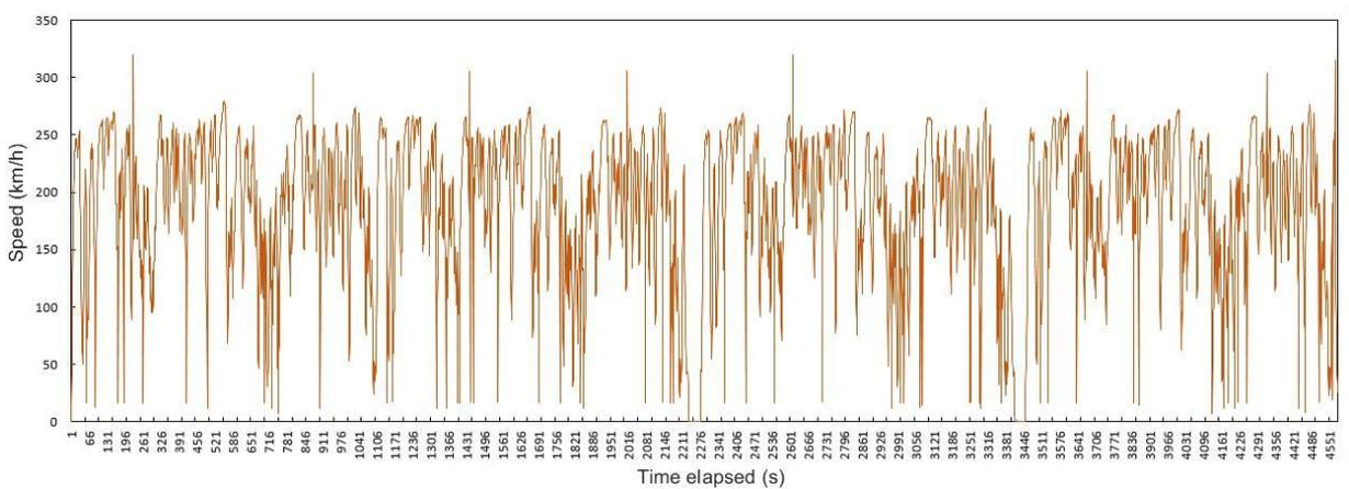
Figure 6.7 - Speed profile generated from sample dashcam video
