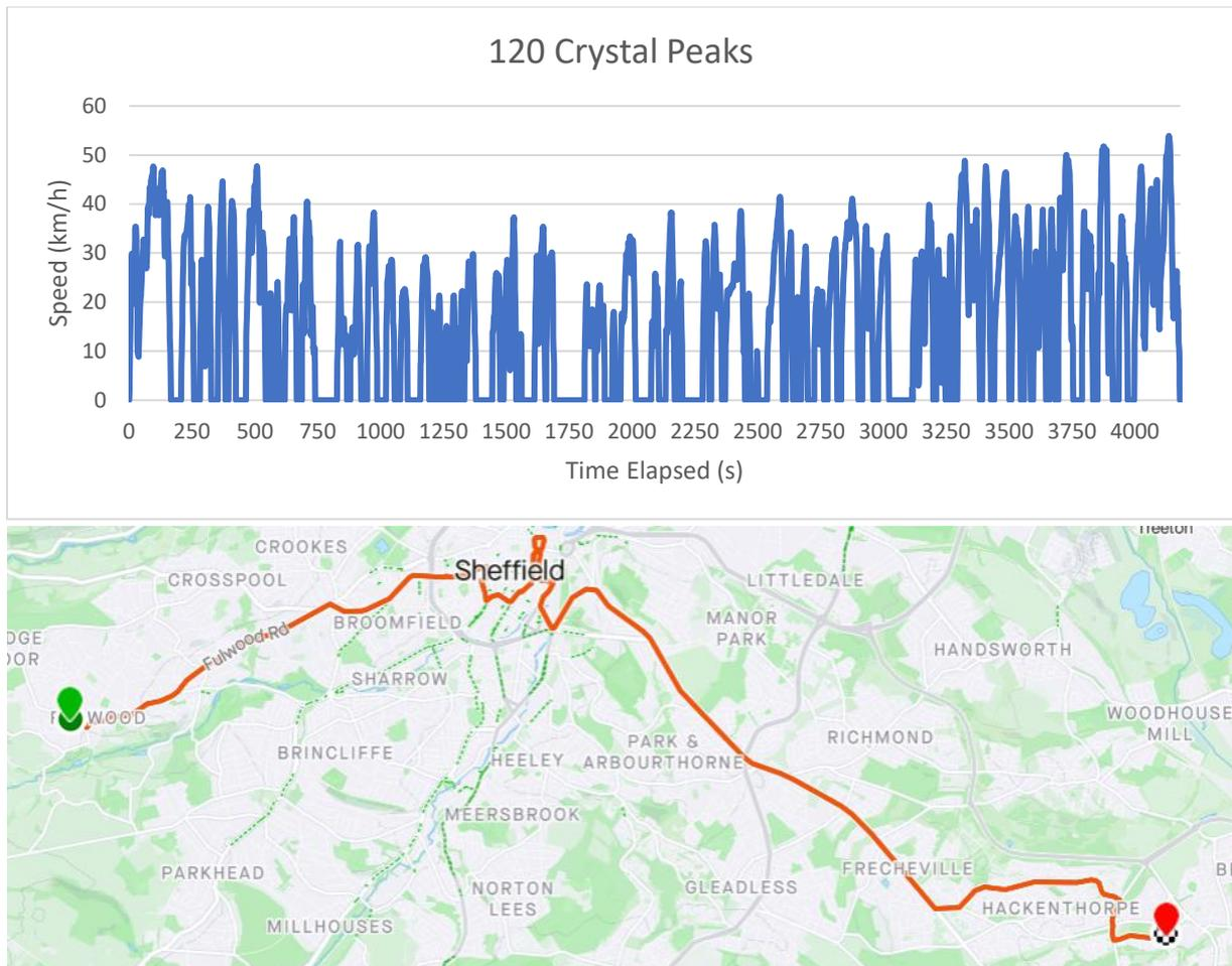
Figure 5.13 - Example of recorded bus telemetry
