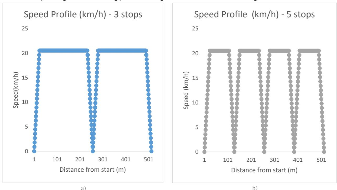
Figure 5.25 - Realistic cycle driving patterns. a) 3 stops, 512m street, 20kph limited, b) 5 stops, 512m street, 20kph limited
