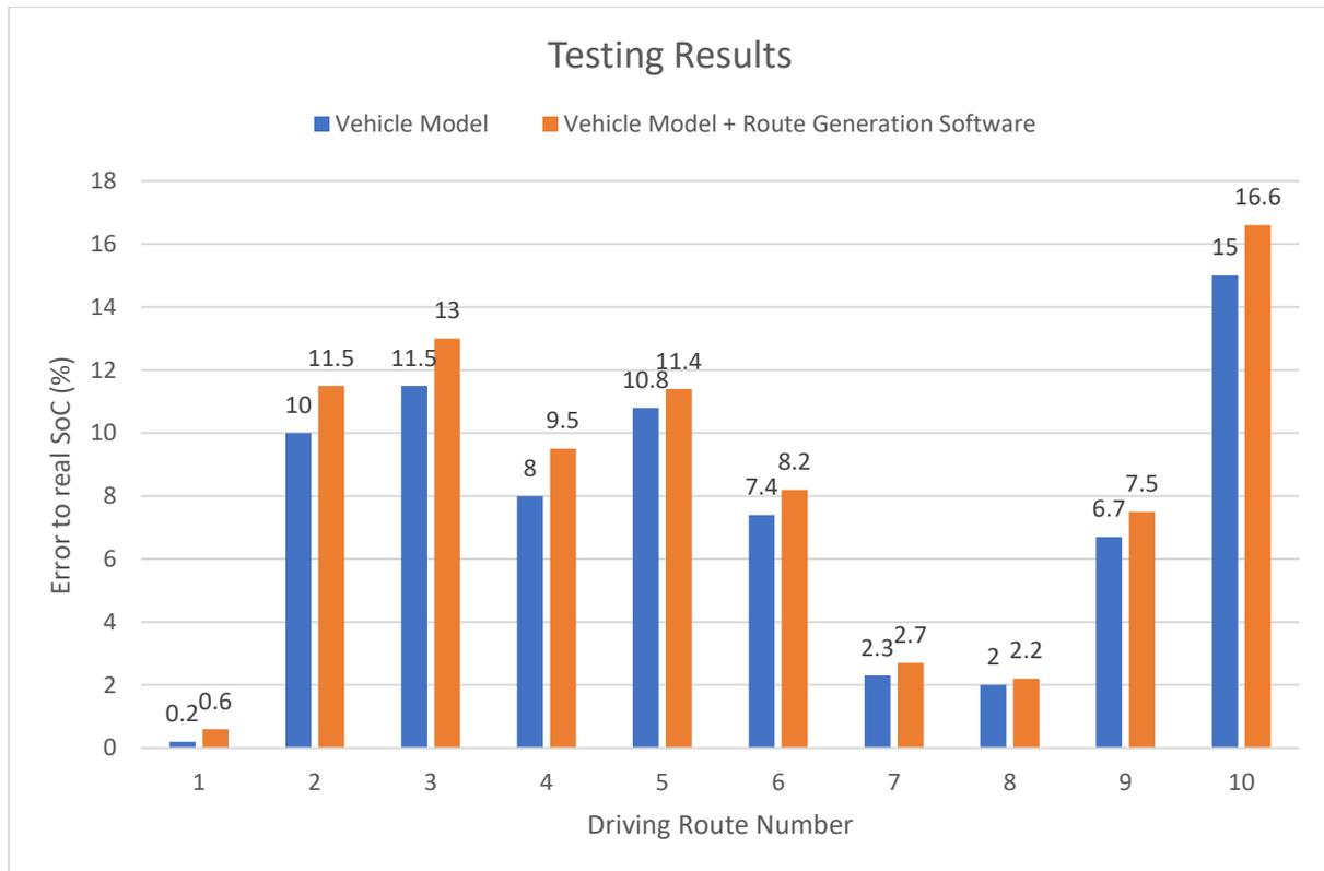
Figure 4.5 - EV model testing results - SoC estimation
