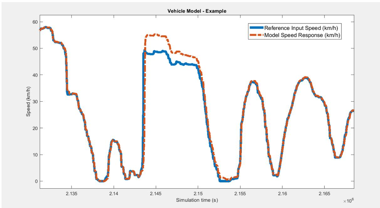
Figure 3.17 - Control module fail (control response overshoot)
