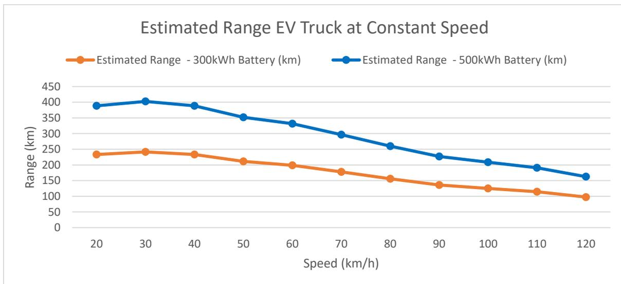
Figure 7.6 - eHGV range curve based on constant energy consumption at various speeds
