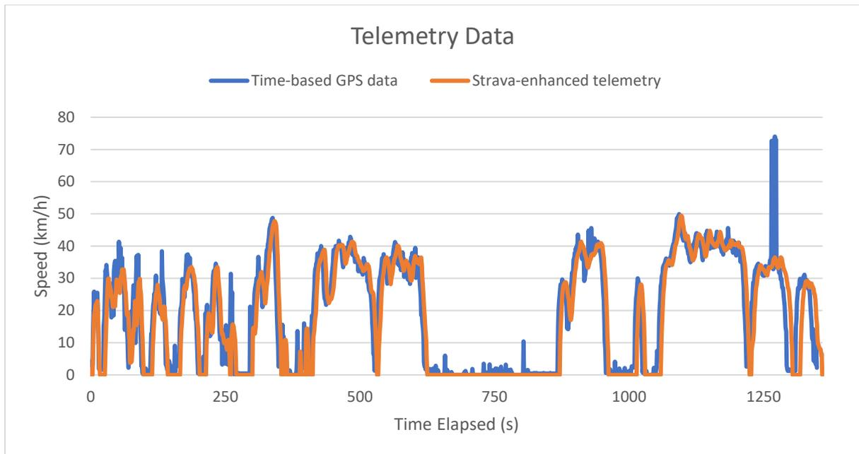
Figure 5.14 - Example of telemetry produced using Strava’s proprietary enhanced speed calculation method and the conventional time-based GPS approach. Note the vehicle idling periods set to zero and the “cleaner” telemetry aspect of the Strava solution (red) relative to the GPS-only information (blue)
