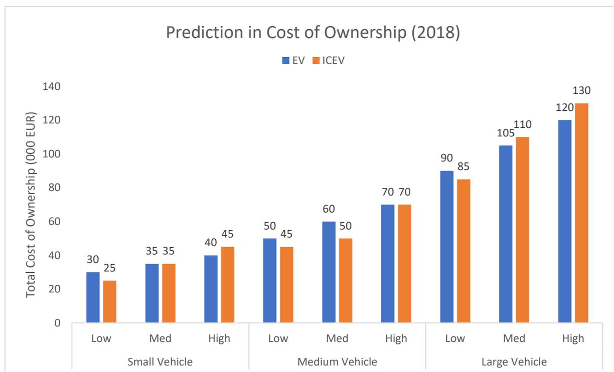
Figure 2.7 - EV cost of ownership prediction [53]. Small/Medium/Large indicates vehicle size and Low/Med/High relates to vehicle use. Total cost of ownership includes energy refuelling, maintenance and taxes.
