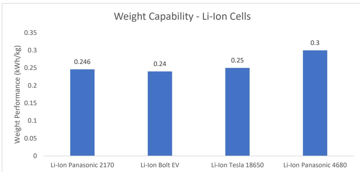
Figure 7.8 - Electrical storage capability with respect to weight [285]
