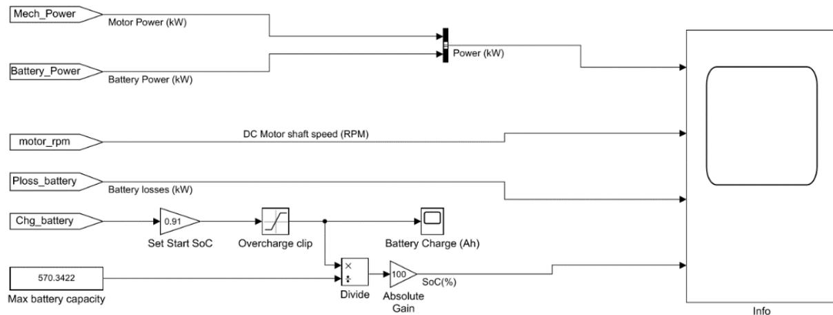
Figure 3.12 - Power information processing subsystem
