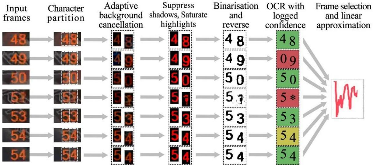
Figure 6.2 - Proposed image processing procedure. Example shows a typical input frame group and its related OCR results with the level of prediction confidence coloured in Green (high), Lime Green (average) and Red (low)
