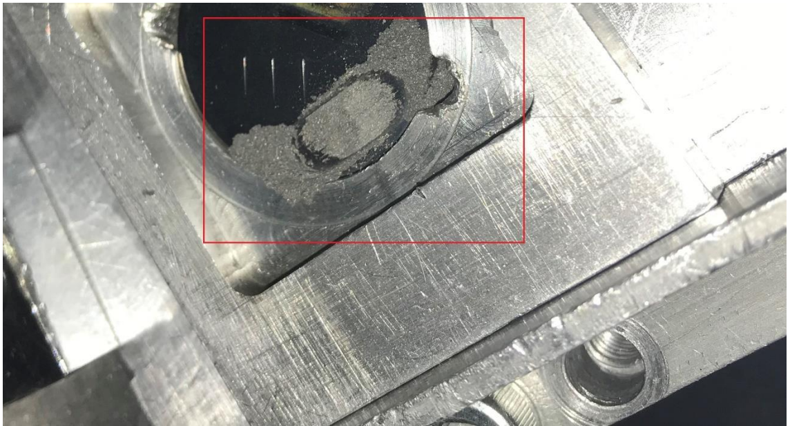
Figure C.1 Delamination of DLC-GNP film under 280N load unlubricated.
