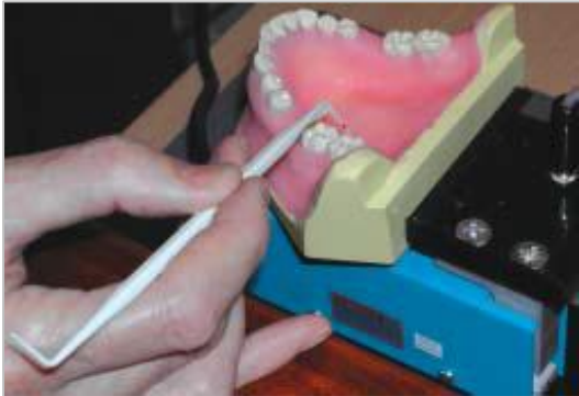
Figure 114. Dental Probe Test apparatus (reproduced from [158])
