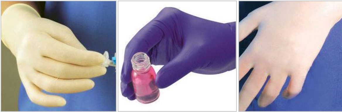
Figure 28. Examination gloves used in testing (a) latex, (b) nitrile and (c) vinyl (reproduced from [159])
