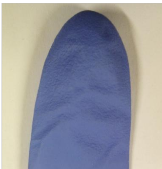
Figure 14. Grip pattern on examination glove fingertips
