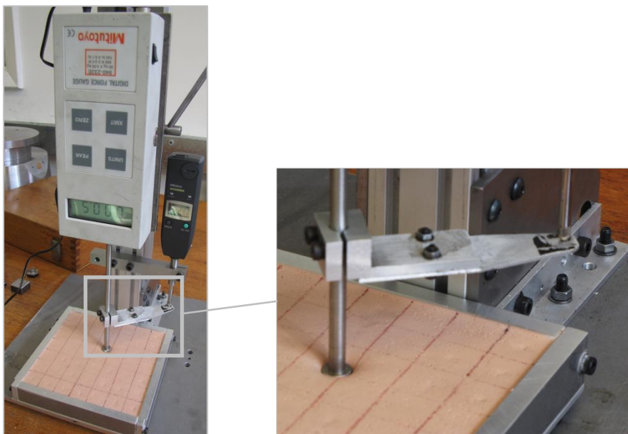
Figure 101. Stiffness testing rig
