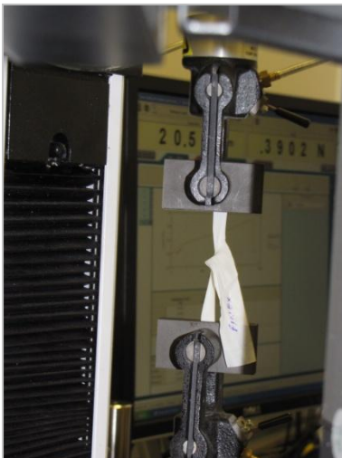
Figure 200. Tear strength test apparatus
