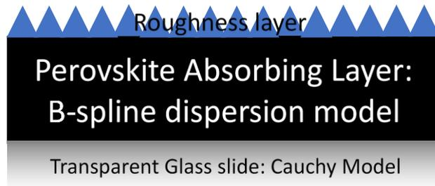
Figure 24: Ellipsometry Model showing glass substrate, perovskite absorber layer, and surface roughness layer assuming 50% void space, 50% perovskite.
