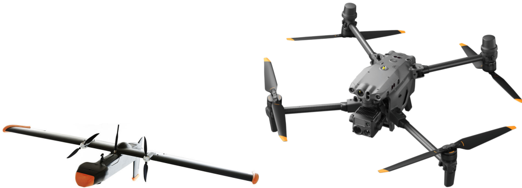
Figure 1.1: UAUVER Avian-P3 commercial fixed-wing UAV ([7]) (Left) and DJI Matrice 30 commercial rotary-wing UAV ([8]) (Right).
