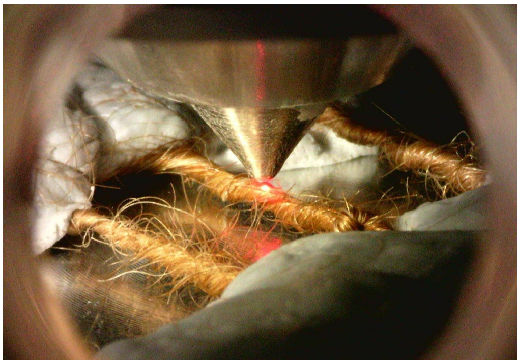
Figure 132: Dog hair samples were twisted into tight bundles for XPS measurements.
