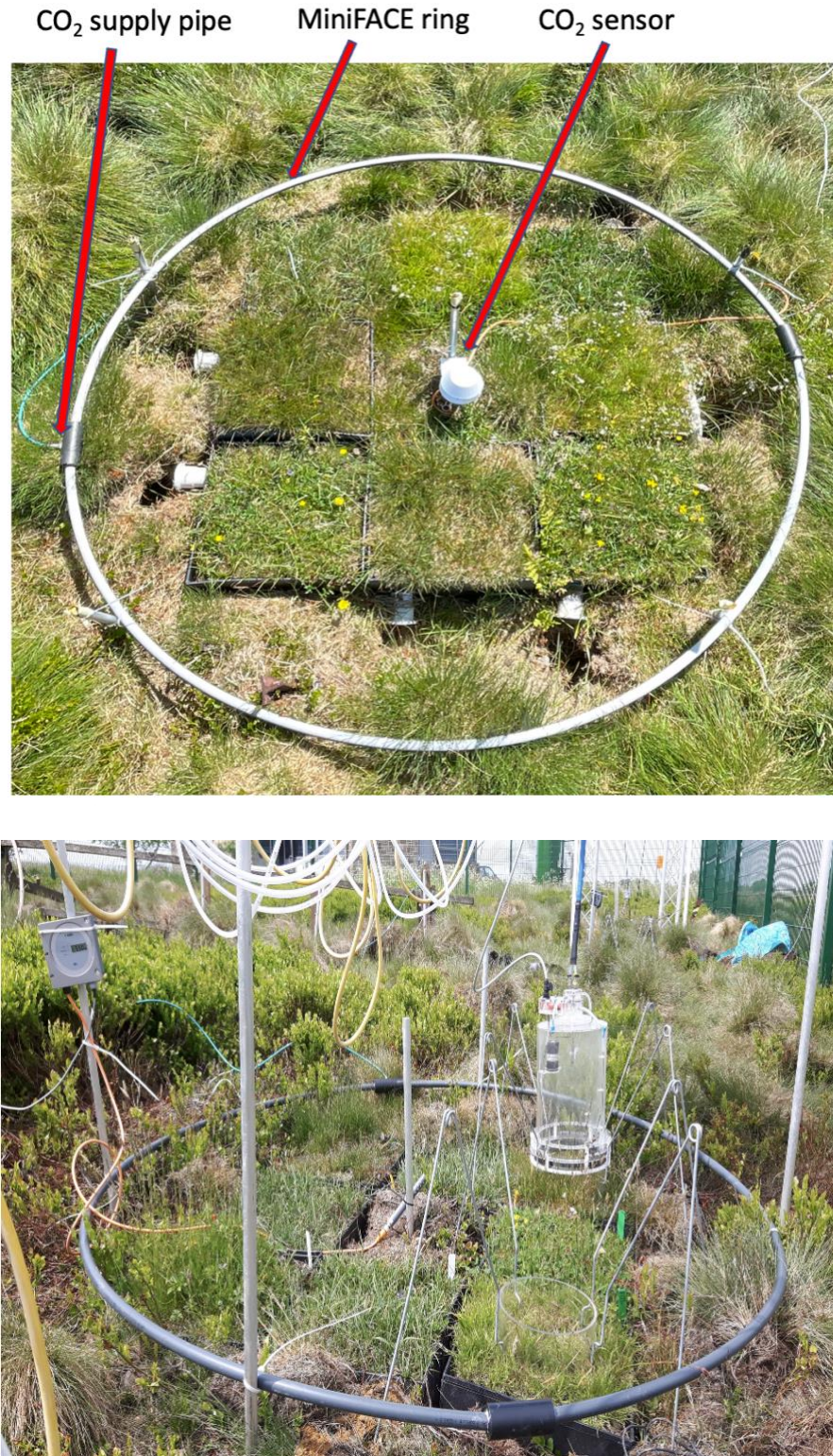
Figure 1.4: The top image of a block of eCO 2 mesocosms. MiniFACE ring with laser-drilled holes provides CO 2 to grasses from a connecting pipe. In order to achieve the target concentration (600 ppm), the central computer receives information from the CO 2 sensor located in the ring's center. This is modified based on the results of a weather station located on the site, considering both the speed and the direction of the wind. The image at the bottom of the page displays an eCO 2 block in the middle of the active experiment, as well as the automated CO 2 flux chamber (Skyline system). Bottom image credit (Ben Keane)
