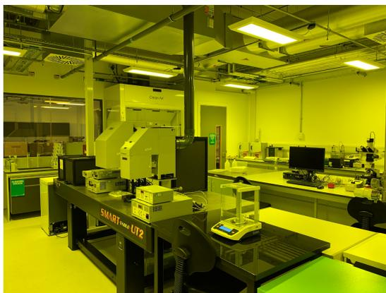
Figure 2.2: Clean room in the Sir William Henry Bragg Building. The gold light is used to ensure photosensitive samples are not exposed to light.
