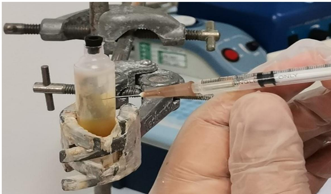
Figure 2.3: Aspiration of lipoproteins. A 19 gauge needle attached to a 1 ml syringe is used to aspirate the different lipoproteins after separation using ultracentrifugation. A 1-2 ml band of LDL was aspirated from each tube and these were pooled and dialyzed in BPS overnight.
