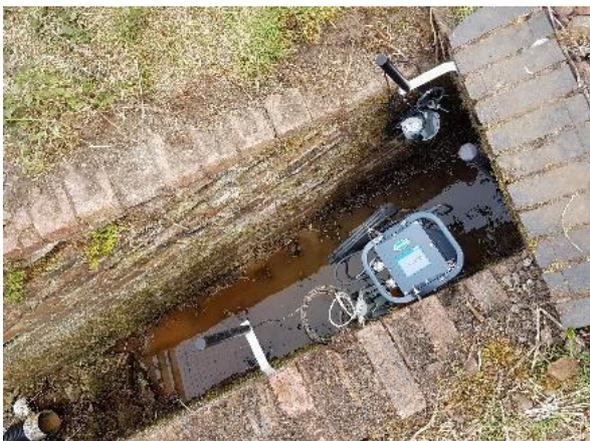
(e) Water depth sensor at culvert entry D1
