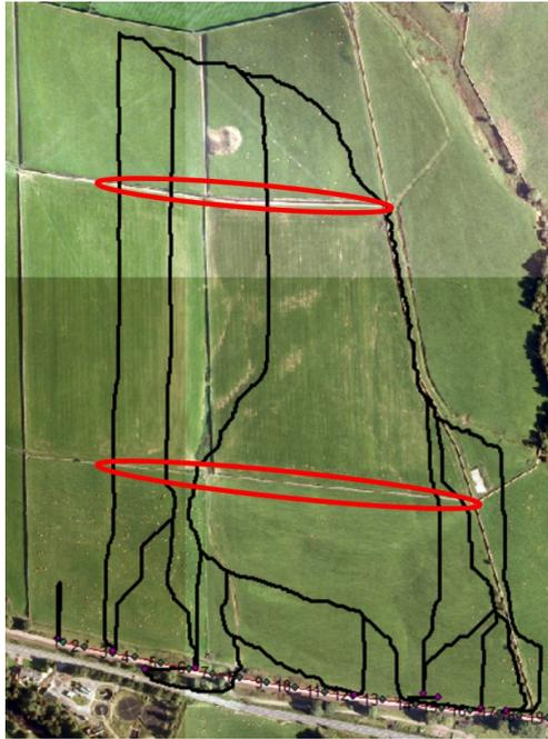
Figure 5.13: Man-made features that could disturb overland flow
