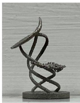
Figure 6.12 A failed sample of the vertical helix design.
