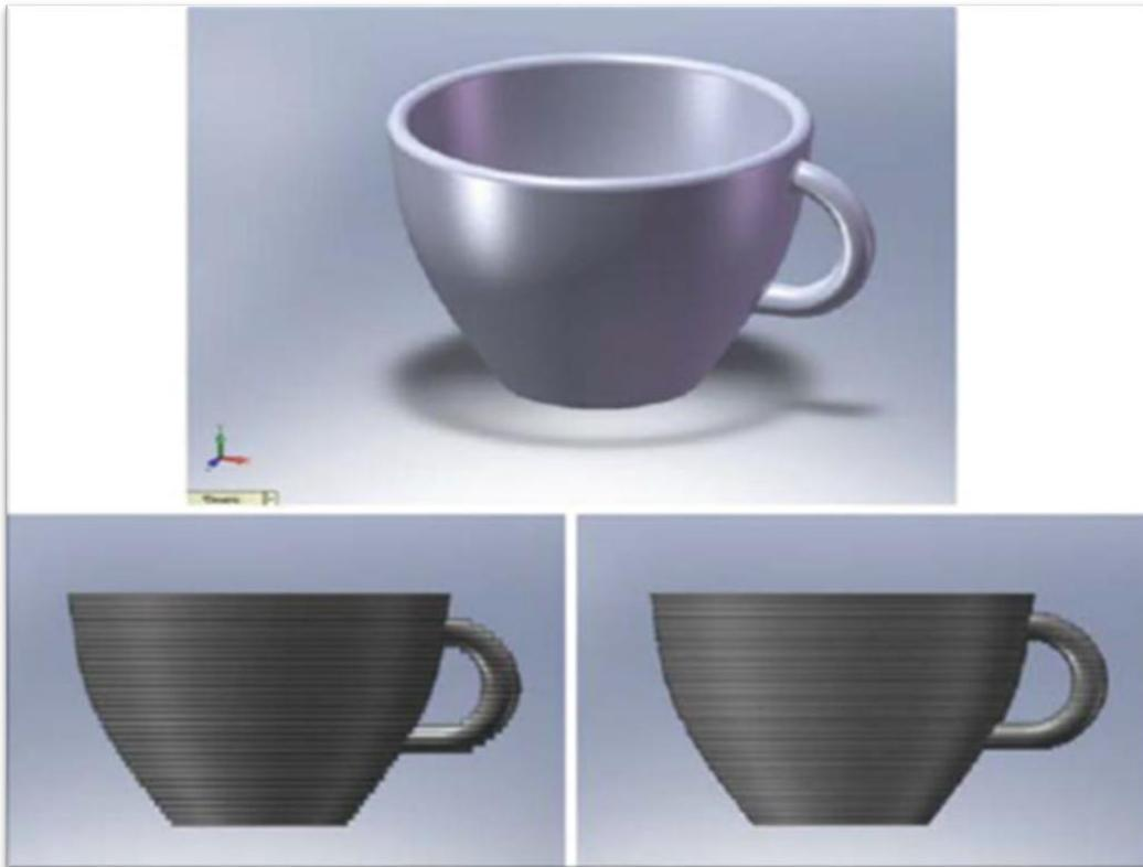
*Figure 2.5 An image illustrating basic AM design or a component (layer by layer) [28].*
