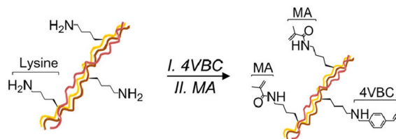
Figure 3.2: Design of functional RTC precursor through sequential functionalisation with both 4-vinylbenzyl chloride (4VBC, I) and then methacrylic anhydride (MA, II) (Modified from (Liang et al., 2022)).
