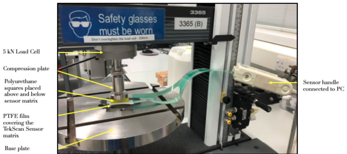
Figure 4.1: Calibration of 5033 TekScan Pressure Sensor Labelled diagram of the calibration method used for the TekScan Pressure Sensor. Polytetrafluoroethylene (PTFE) tape was used to reduce incidence of sensel drop out during testing and thus was included during calibration.
