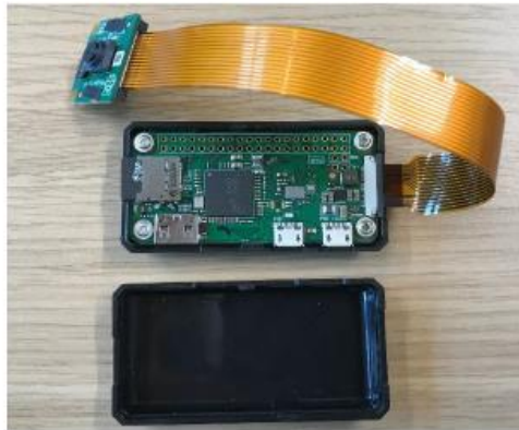
Figure 1. One Raspberry Pi camera unit with v2 camera, RPi zero CPU and casing
