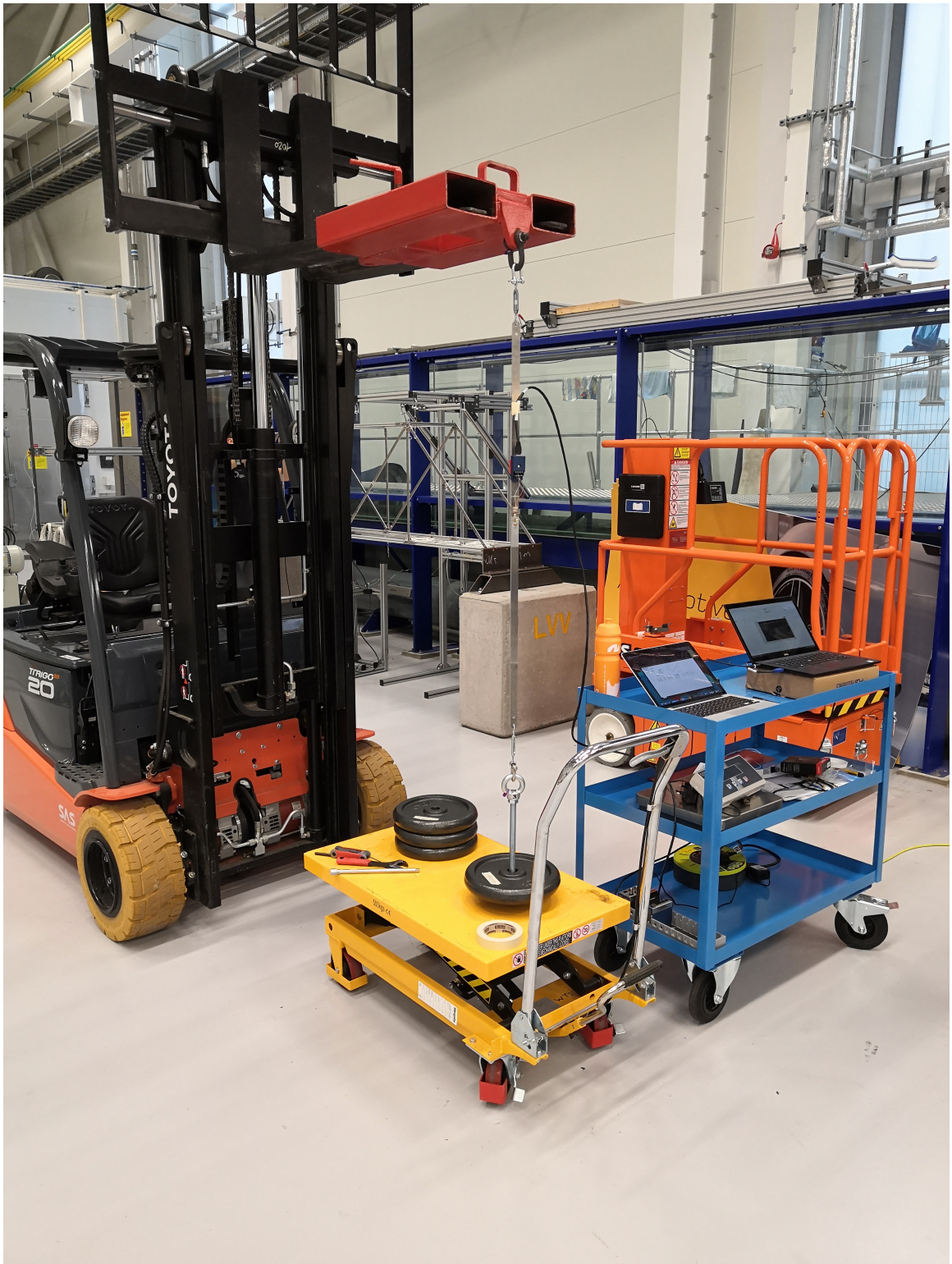
Figure A.5: The rig used for strain gauge calibration
