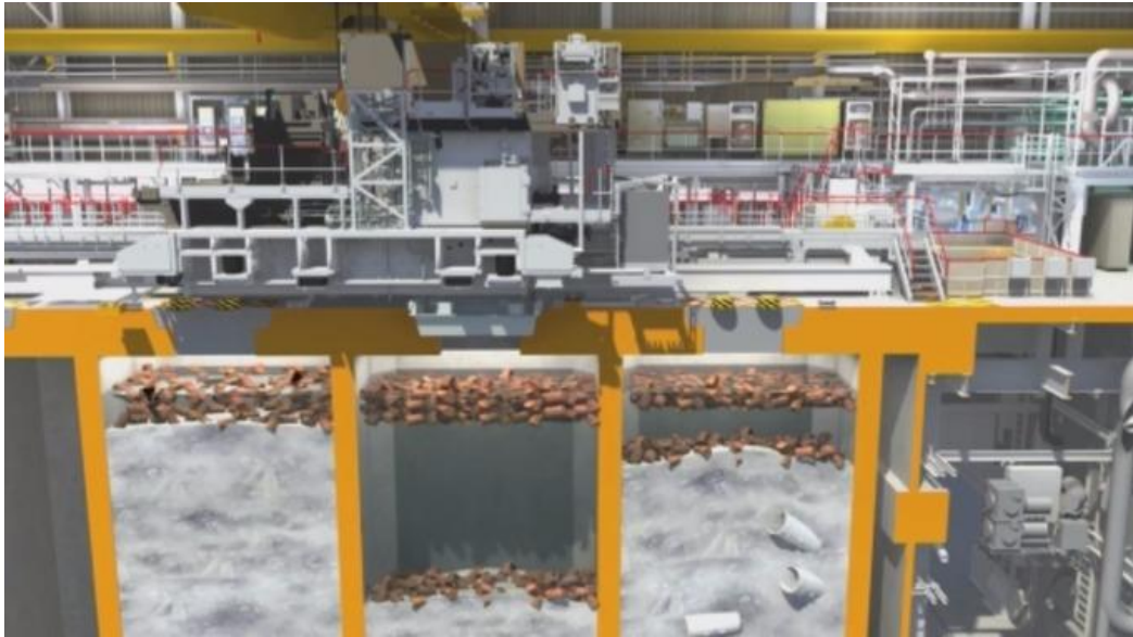
Figure 2.1 Magnox swarf storage silo, cross section (RadioRoSo, 2022)
