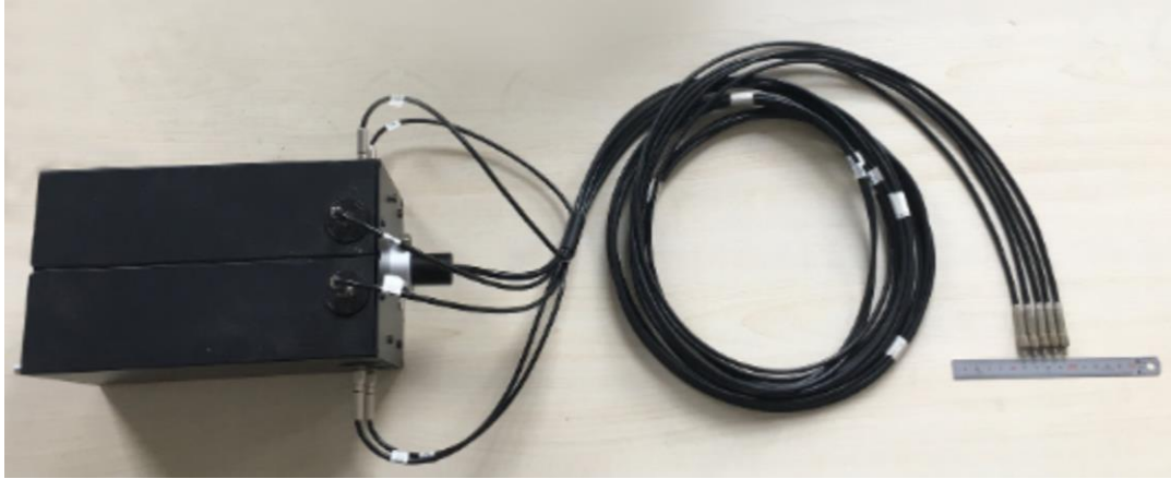
Figure 2.6 Five-channel miniature optical fibre sediment concentration measuring instrument (Huang and Zhang, 2021)
