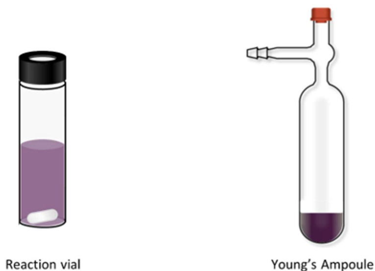
Figure 3.3 – Illustration of the vial and the ampoule for use in the catalytic studies. An inert atmosphere was provided by an Ar inlet needle for the vial, and an Ar line attached to the side inlet for the ampoule.
