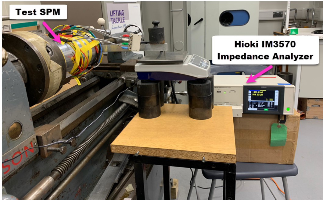
Fig. 7.7 Inductance measurement by the Hioki IM3570 Impedance Analyzer.
