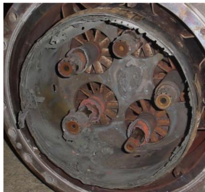
Fig. 1.2. Destroyed combustor structure due to the unexpected thermoacoustic oscillations [4].
