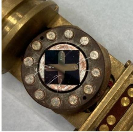
Figure 6.1: A typical sample with cross-shaped geometry, wirebonded for measurement of the longitudinal and transverse resistance of the sample.
