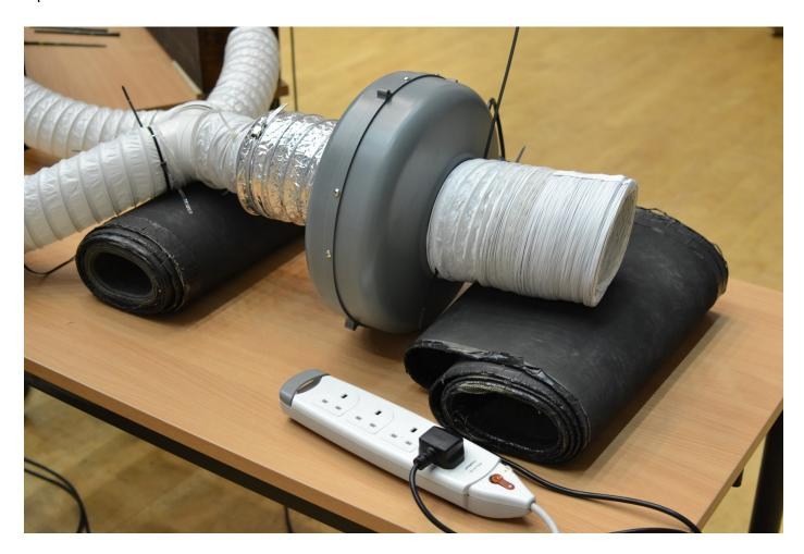
In order to achieve an air-tight seal between the sections of ducting hose and each pipe, you will require ducting adapters to allow the 4" hose to connect to the foot (air intake nozzle) of each pipe. Alternatively, you may remove the foot of each pipe, and insert ducting adapters directly into each pipe — remember to use electrical tape and duct tape where necessary to achieve air-tight seals (see photograph on next page).
