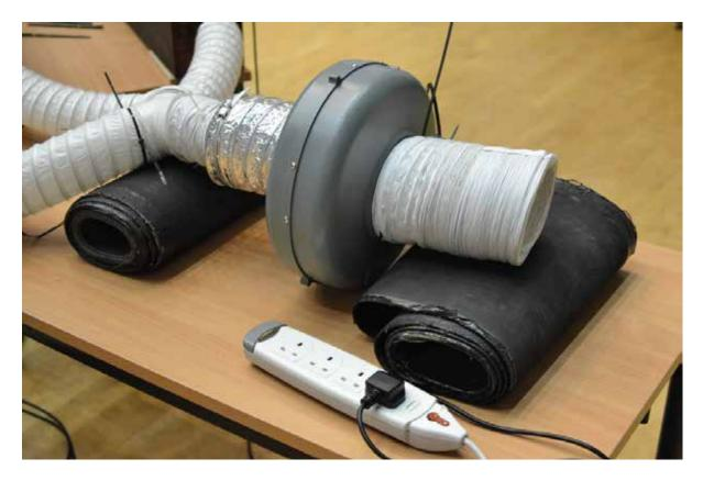
In order to achieve an air-tight seal between the sections of ducting hose and each pipe, you will require ducting adapters to allow the 4" hose to connect to each pipe toe. Alternatively, you may remove the air intake nozzle on each pipe, and insert ducting adapters directly into each pipe—remember to use electrical tape and duct tape where necessary to achieve air-tight seals (see photograph on next page).
