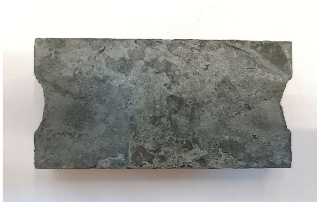
Figure 74 PSC sample after the heat treatment, the sample was processed at 1300°C and 5°C/s of cooling rate.
