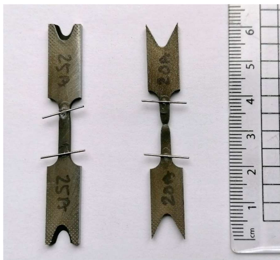
Figure 77 Tensile sample before and after the test, the scale is represented in centimetres.
