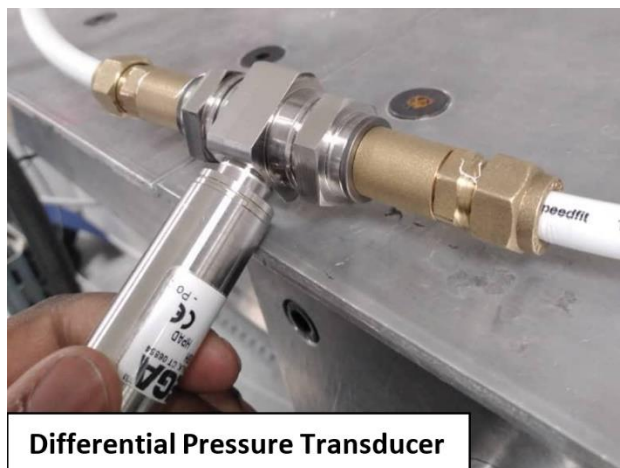
Figure 3.16: Omega PX409 series wet/wet differential pressure transducer connected to the computer showing pressure readings
