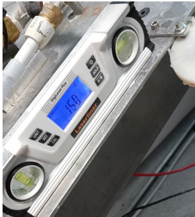
Figure 3.22: Digital inclinometer used to measure the rigs inclination
