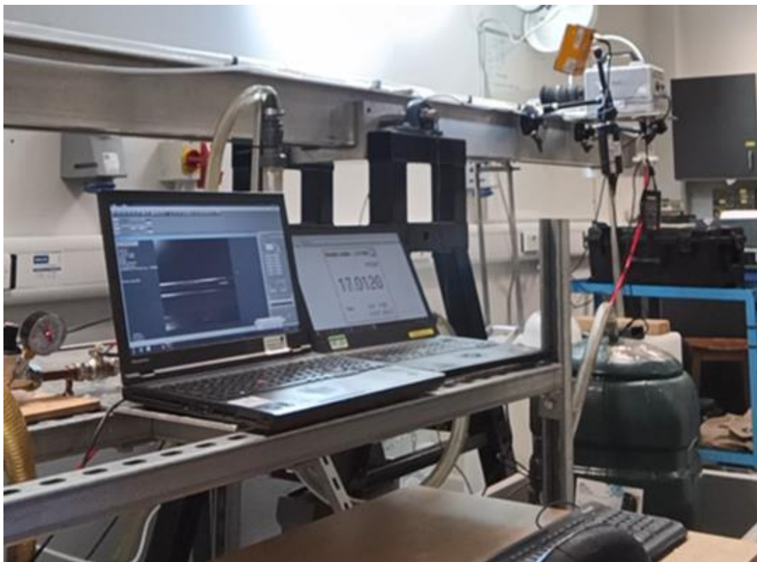
Figure 3.23: Flow visualisation and pressure drop logging station
