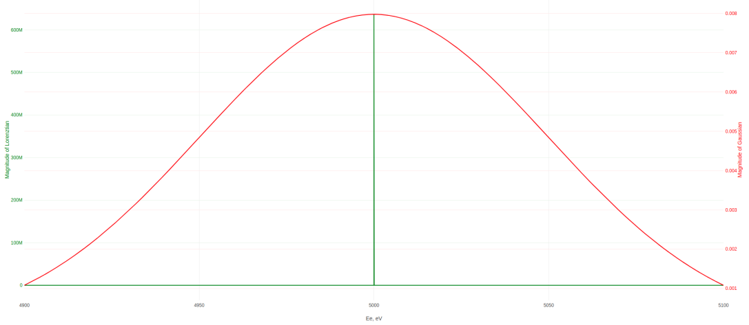
FIGURE 3.3: Magnitude of a Gaussian (red) and Lorentzian function (green) with the same energy axis, for a typical EBIT electron beam longitudinal width and a ^{57}\text{Fe}(0)\text{N}0 capture to excite the 14keV Mossbauer transition E_e = 5\text{keV} . The y axes are adjusted so their peaks match in height, so the green area also shows the resonant fraction for a normalised Gaussian
