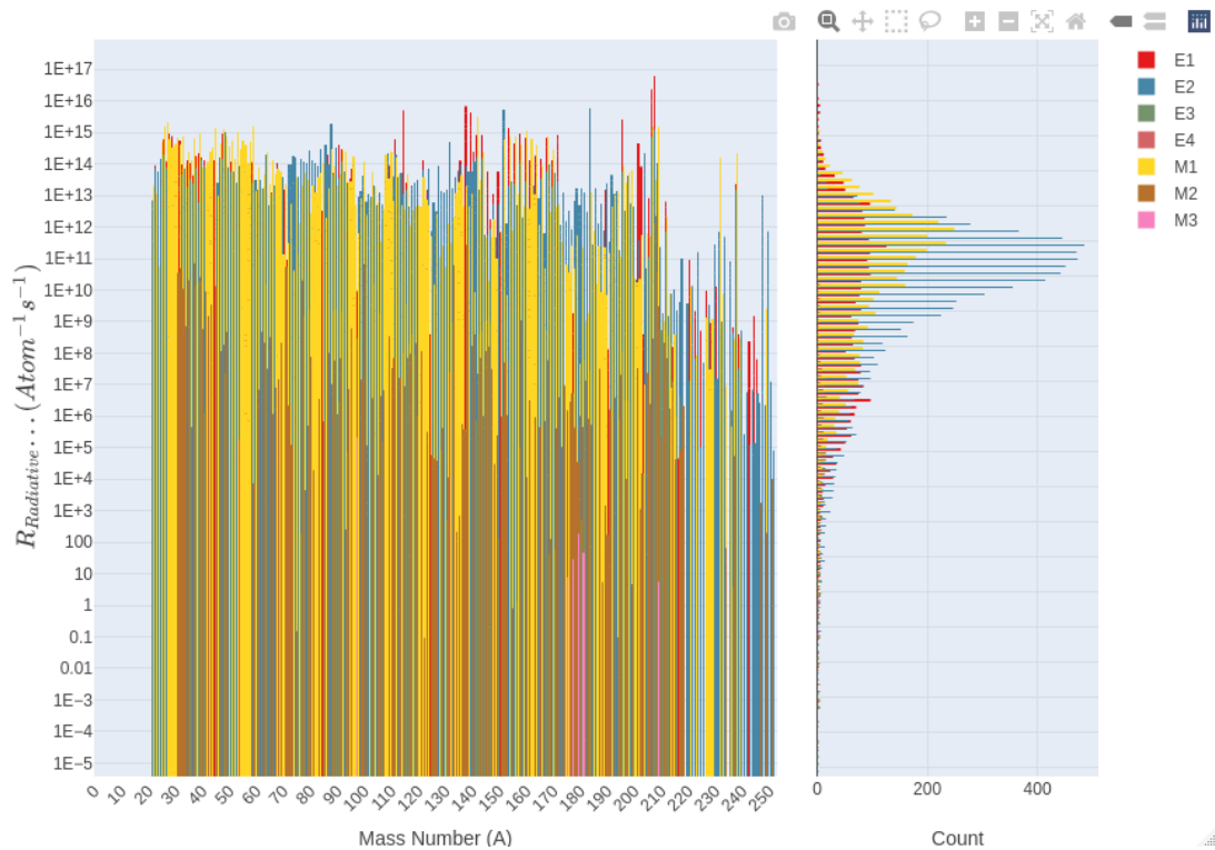
FIGURE 4.6: All of the radiative transition rates R_{radiative} = A_r (per atom per second) with negligible rates discounted, using all ENSDF gamma ray data with known matrix elements. Left: All rates plotted across mass number. Right: data from the left projected onto an aligned histogram in A_r . There are \sim 17,000 nuclear transitions in this dataset, with there being of course no restriction on the resultant state after photon emission
