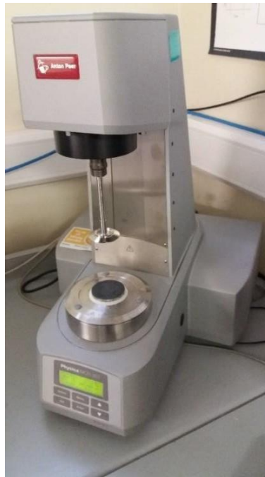
Figure 4.6: Anton Paar Physica MCR 301 with a 50mm plate-plate measuring system attached in the raised position.
