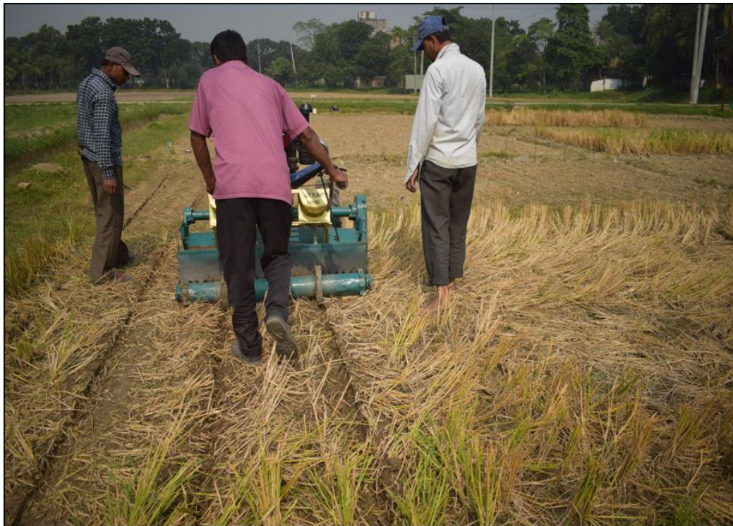
Figure 1.4: A Versatile Multi-Crop Planter is used for strip tillage. Adapted from experimental plot, November 2019.
