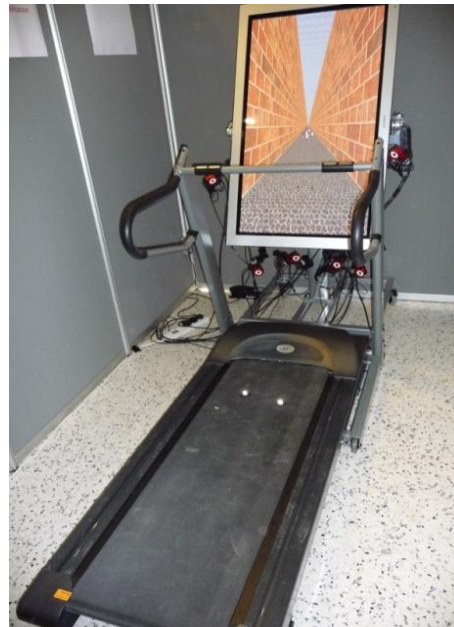
Figure 3.13 StroMoHab was configured based on the design option 3. Cameras were all mounted on the virtual reality display and looking forward to the treadmill, markers were put at the front of the treadmill.
