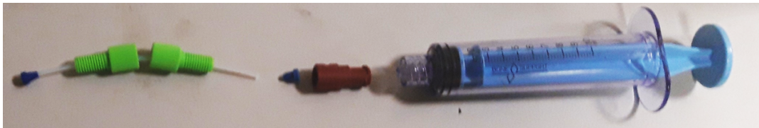
FIGURE 4.35: Attachment of the fluidic part to the syringe.
